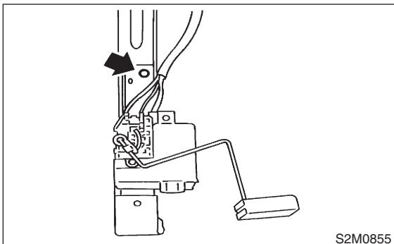
(4) Connect connector to fuel pump relay.
