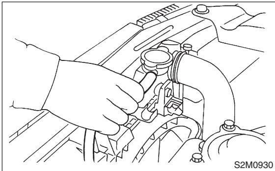
2) Remove bolts which install reservoir tank onto radiator main fan shroud.
