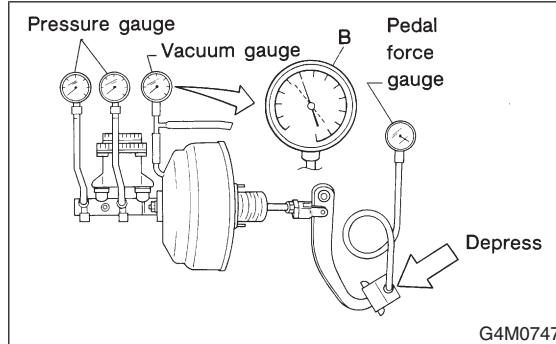
2) Stop engine and watch vacuum gauge. If the vacuum drop range is less than 3.3 kPa (25 mmHg, 0.98 inHg) within 15 seconds after stopping engine, brake booster is functioning properly. If defective, refer to "Air tightness check". <Ref. to BR-44 INSPECTION, Brake Booster.>
