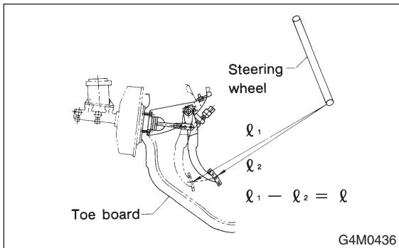
**Specified pedal stroke:****Without ABS****90 mm (3.54 in)****With ABS****95 mm (3.74 in)****When depressing brake pedal with a 490 N (50 kg, 110 lb) load.**
