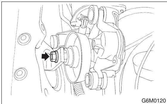
4) Remove nuts which secure sleeve unit.
