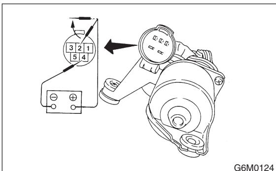
4) Reconnect battery and ensure that wiper motor stops at "AUTO STOP" after operating at low speed.
