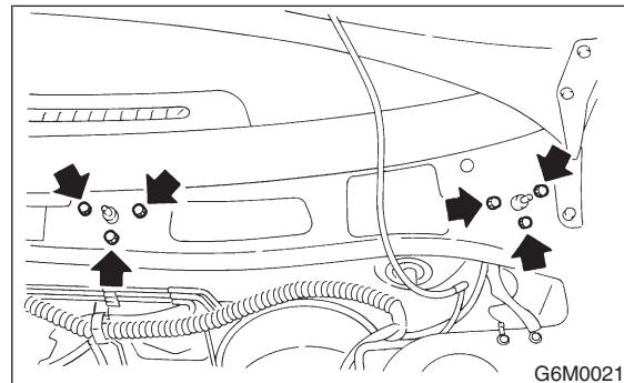
5) Remove wiper link from service hole in front panel.
