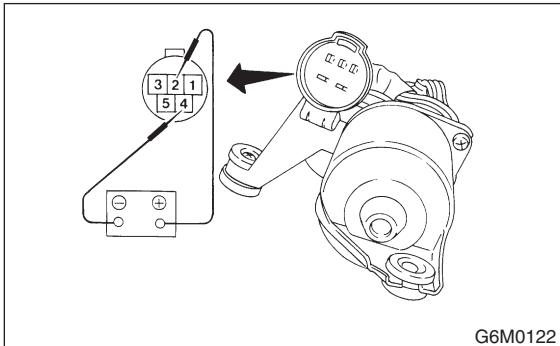
2) Check wiper motor operation at high speed:
