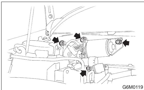
3) Remove nut securing motor link on the back side of motor.
