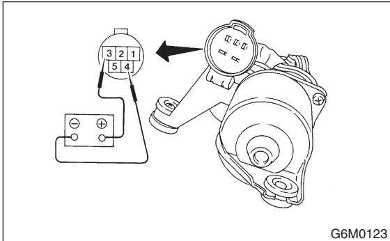
3) Check wiper motor for proper stoppage:
