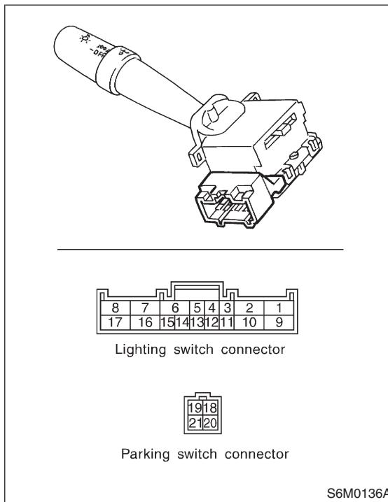
Move combination switch to respective positions and check continuity between terminals.
