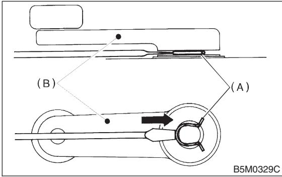
2) Using ST, disengage the clip.
