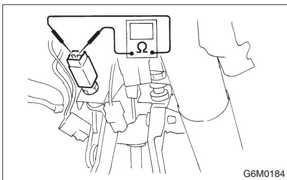
Check continuity between clutch switch terminals.
