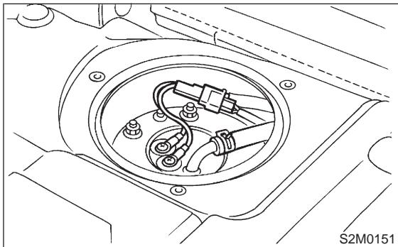
6) Remove bolts which install sub fuel level sensor on fuel tank.
