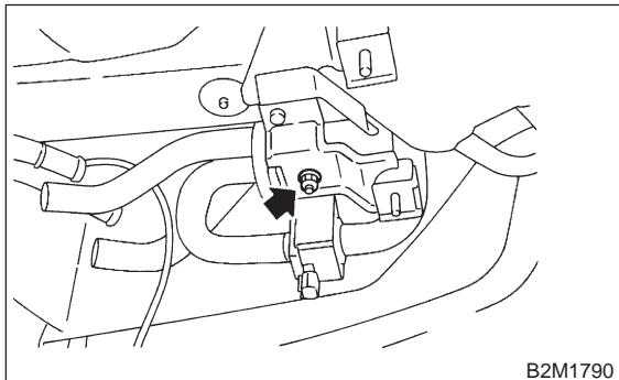
7) Disconnect evaporation hoses, and remove air filter.
