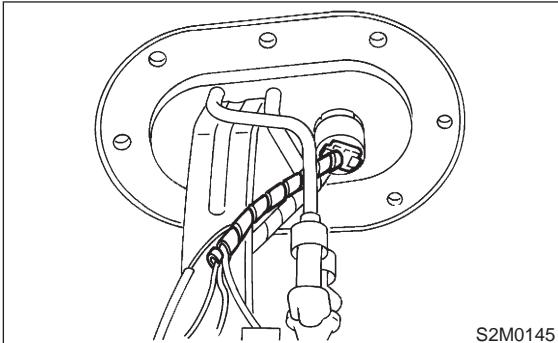
10) Remove main fuel level sensor from fuel pump assembly. <Ref. to 2-1 [W8A0].>
