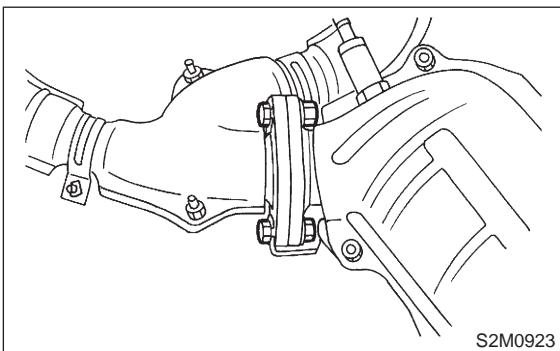
3) Install front exhaust pipe to cylinder heads.
