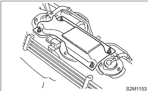
7) Move clips, and disconnect hoses from vent valve.
