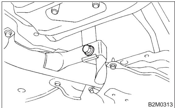
6) Connect rear oxygen sensor connector.
