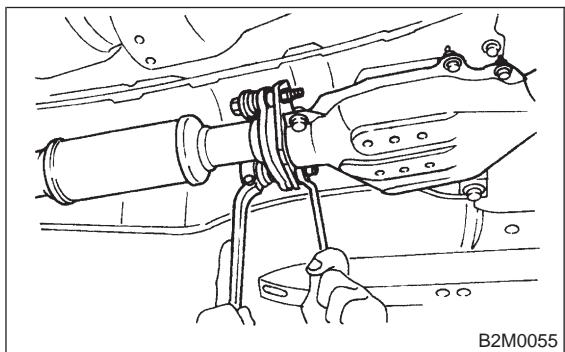
5) Tighten bolt which holds front and rear catalytic converter assembly to hanger bracket.
