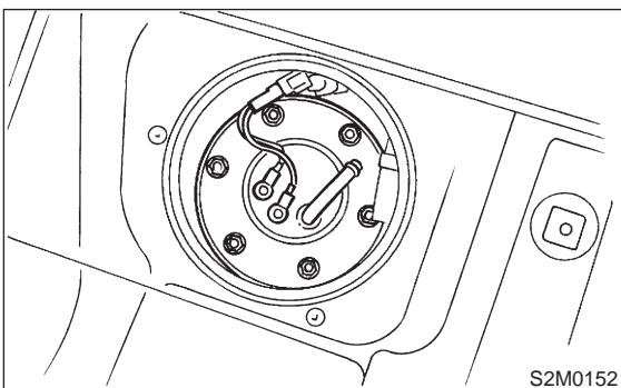
7) Remove sub fuel level sensor.
