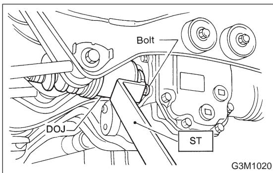
13) Remove DOJ of rear drive shaft from rear differential using ST. <Ref. to 3-4 [W3A2].>
