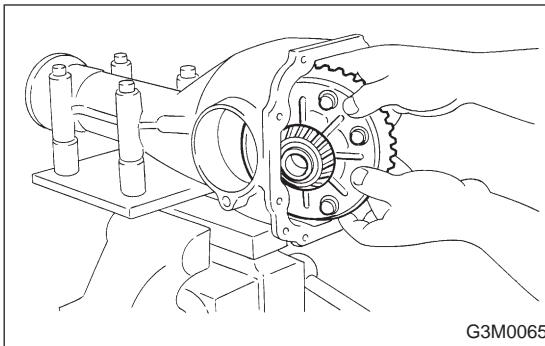
7) Pull out differential assembly from differential carrier.
