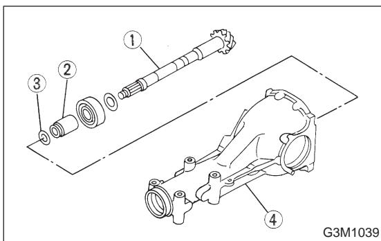
5) Insert drive pinion ① into differential carrier ④, install the previously selected bearing preload adjusting spacer ② and washer ③.
