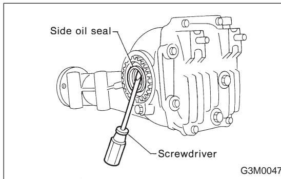
10) Remove oil seal with screwdriver.
