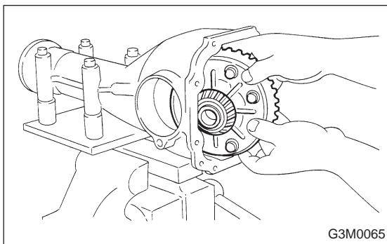
(3) Install the differential case assembly into differential carrier in the reverse order of disassembly.
