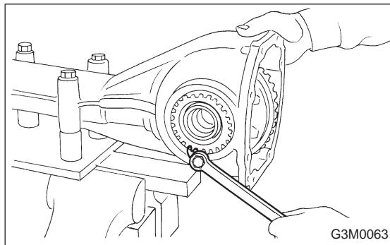
(5) Temporarily tighten lock plate.
