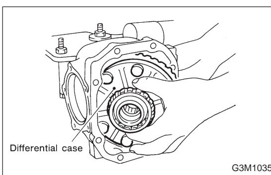
6) Pull out differential assembly from differential carrier.
