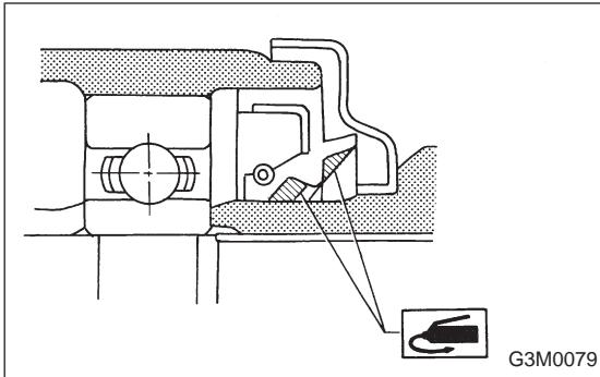
(7) Replace the oil seal with new one at every disassembly. Apply chassis grease between the lips when installing the oil seal.
