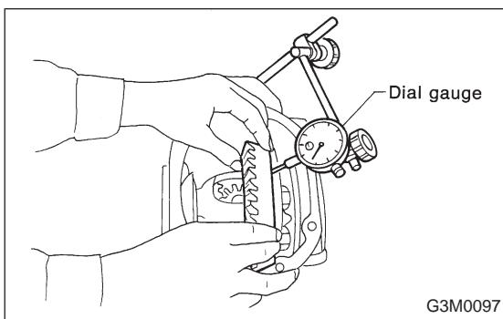
18) Check the crown gear runout on its back surface, and make sure pinion and crown gear rotate smoothly.
