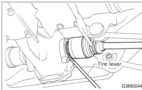
(7) Remove the DOJ from the rear differential with tire lever.
