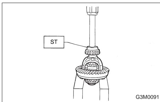
14) Press side bearing cone onto differential case with ST1.
