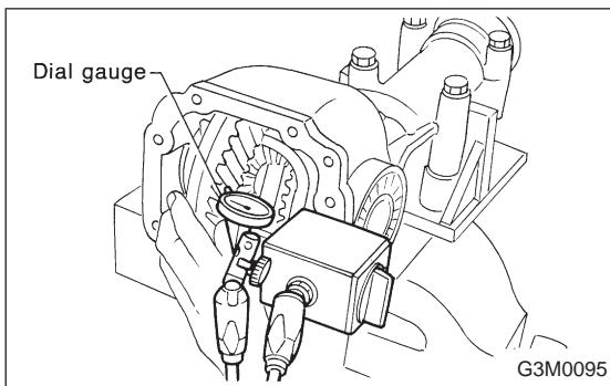
17) Re-check crown gear-to-pinion backlash.
