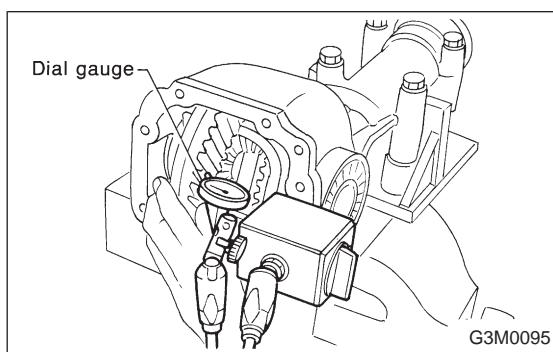
(6) Measure the crown gear-to-drive pinion backlash.
