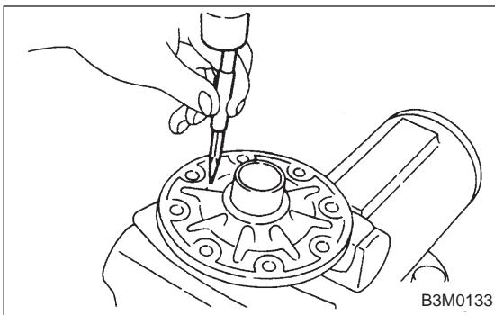
12) Drive out pinion shaft lock pin from crown gear side.
