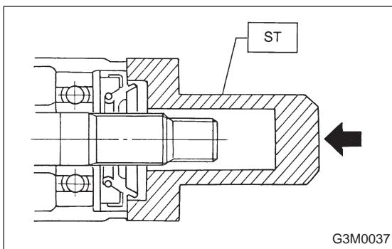
10) Fit a new oil seal using ST.
