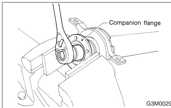
3) Place companion flange in a vise and remove stake nut.
