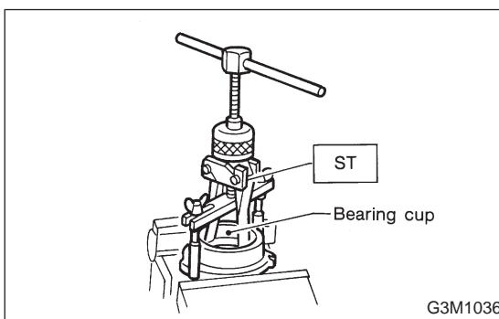
7) When replacing side bearing, pull bearing cup from side bearing retainer using ST.
