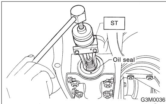
9) Remove oil seal using ST.
