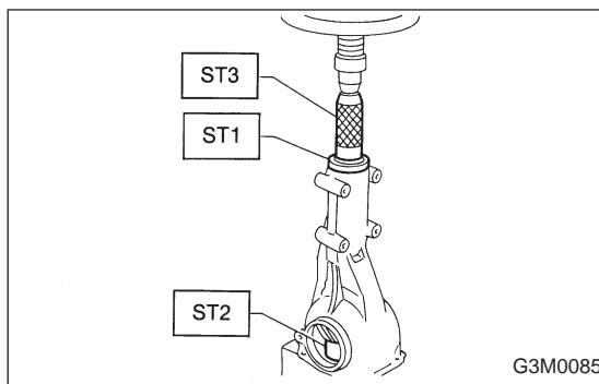
6) Press-fit front bearing cone into case with ST1, ST2 and ST3.
