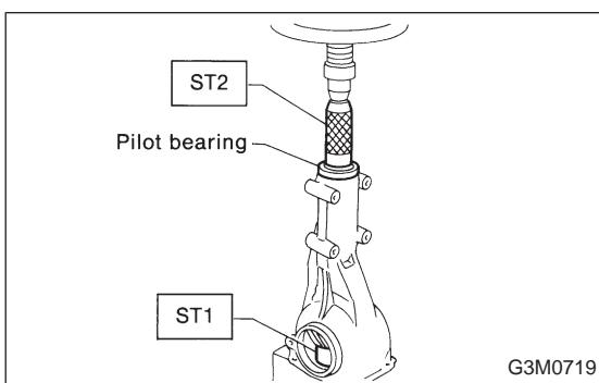
7) Insert spacer, then press-fit pilot bearing with ST1 and ST2.
