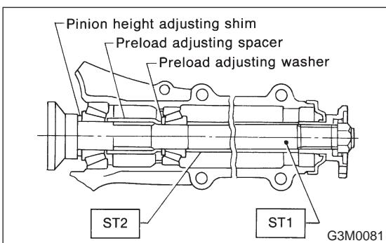
(4) Insert ST1 into case with pinion height adjusting shim and rear bearing cone fitted onto it.
