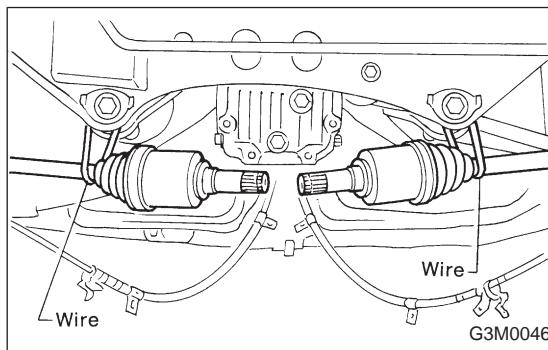
9) Secure rear drive shaft to rear crossmember using wire.
