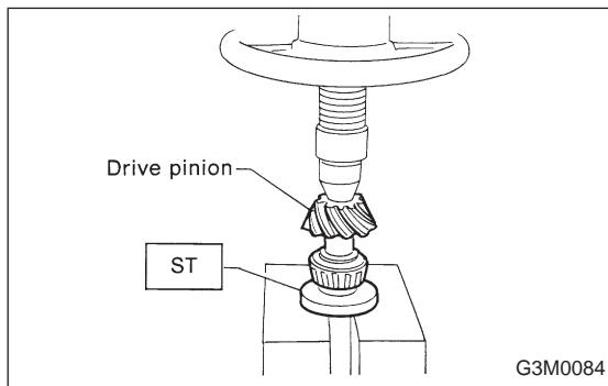
4) Install the selected pinion height adjusting shim on drive pinion, and press the rear bearing cone into position with ST.
