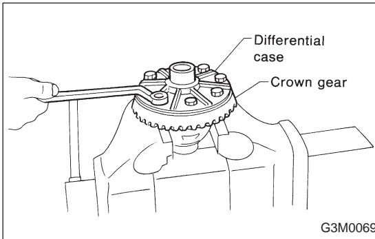
11) Remove crown gear by loosening crown gear bolts.
