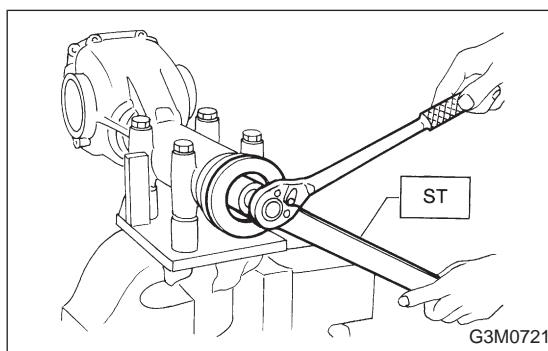
10) Install self-locking nut. Then tighten self-locking nut with ST.
