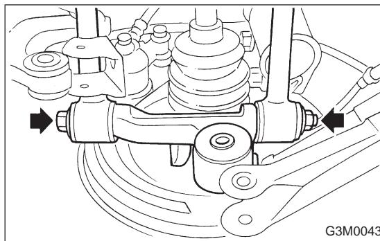
(6) Remove the bolts which secure the front and rear lateral link to the rear housing.
