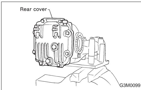
21) Install rear cover and tighten bolts to specified torque.
