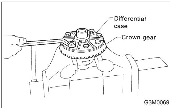
12) Install crown gear on differential case.
