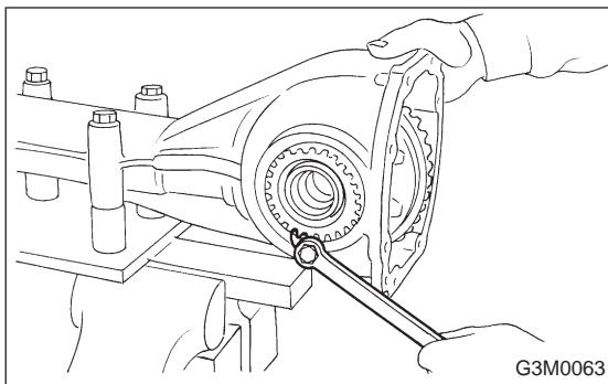
16) Tighten bolt of lock plate to specified torque.
