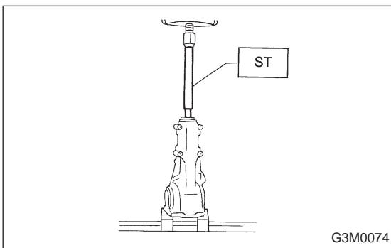
16) Press the end of drive pinion shaft and extract it together with rear bearing cone, preload adjusting spacer and washer.
