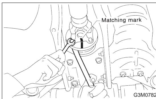
2) Align matching marks and connect flange yoke and rear differential.
