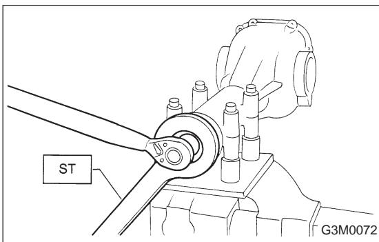
14) Hold companion flange with ST and remove drive pinion nut.
