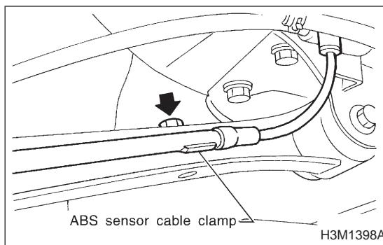
(2) Remove the ABS sensor cable clamp from the trailing link.
