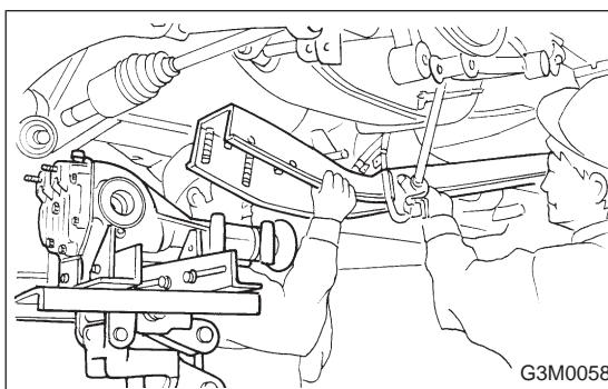
19) While slowly lowering transmission jack, move rear differential forward and remove bolts from rear crossmember.
