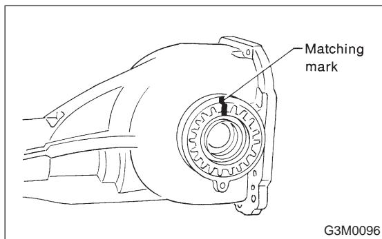
15) Draw a matching mark on both differential carrier and holder. Remove holder one side at a time.
