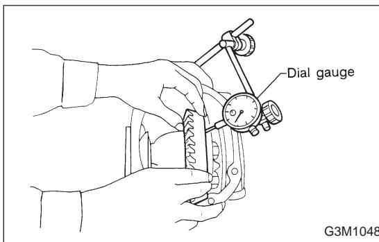
16) Re-check crown gear-to-pinion backlash.
