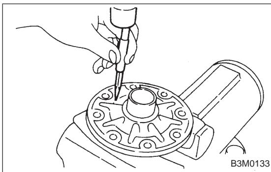
10) Drive out pinion shaft lock pin from crown gear side.
