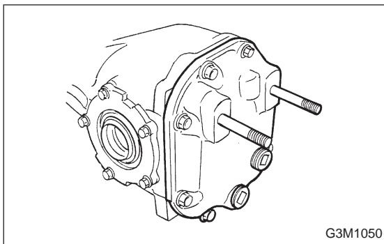
20) Install rear cover and tighten bolts to specified torque.
