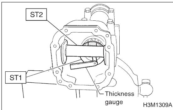
(2) Measure the clearance N between the end of ST2 and the end surface of ST1 by using a thickness gauge.
