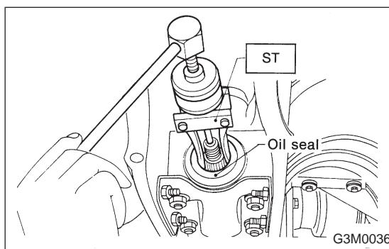
9) Remove oil seal using ST.
