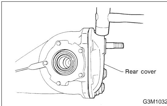
4) Remove rear cover by loosening retaining bolts.
