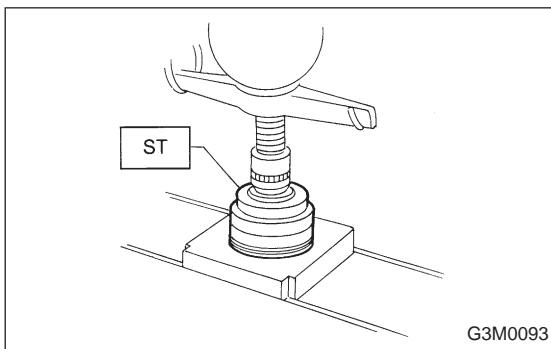
(2) Install bearing race into right and left holders.
