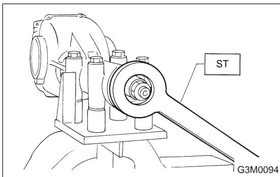
14) Perform adjustment of backlash of pinion crown gear set and adjustment of preload of differential side bearing.
