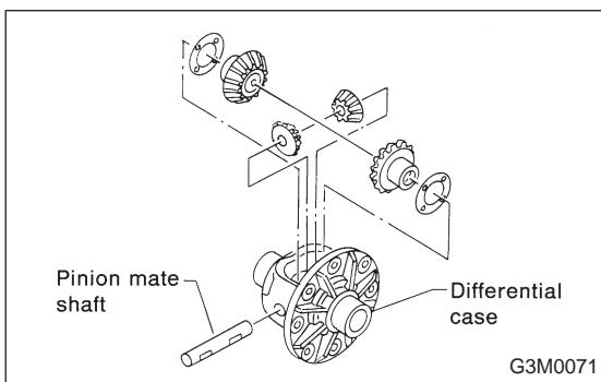
11) Draw out pinion mate shaft and remove pinion mate gears, side gears and thrust washers.
