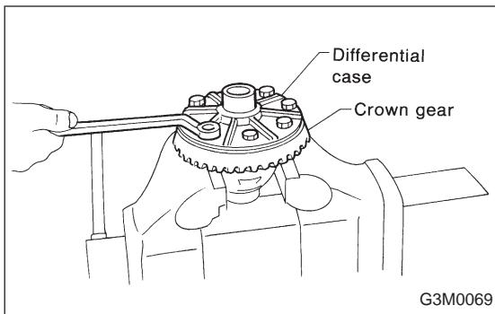
9) Remove crown gear by loosening crown gear bolts.
