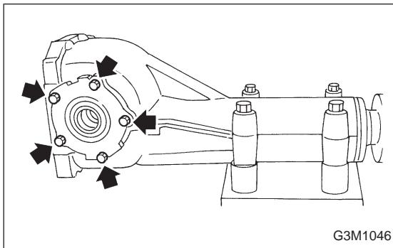
(5) Tighten side bearing retainer bolts.
