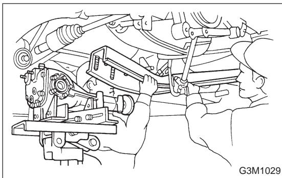
20) While slowly lowering transmission jack, move rear differential forward and remove front member and rear differential from body.
