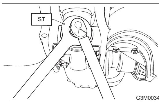
7) Remove self-locking nut while holding companion flange with ST.
