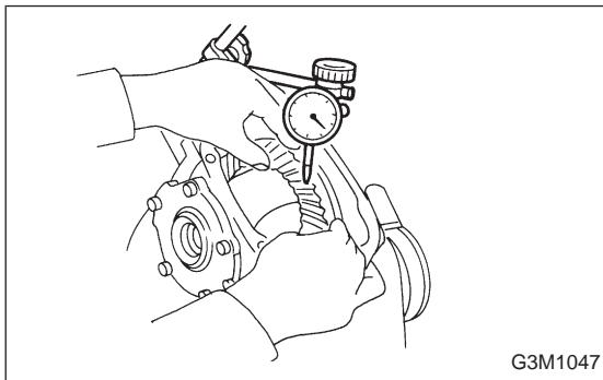
(6) Measure the crown gear-to-drive pinion backlash.
