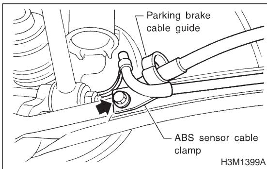
(3) Remove the ABS sensor cable clamp and parking brake cable guide from the trailing link.
