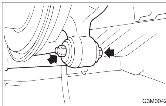
(5) Remove the bolts which secure the trailing link to the rear housing.
