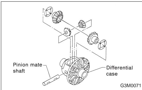
13) Draw out pinion mate shaft and remove pinion mate gears, side gears and thrust washers.
