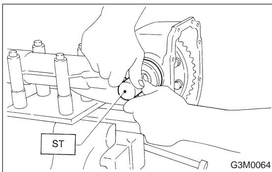
(2) Screw in side (left-side) holder until light contact is made with ST.
