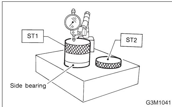
13) Before installing side bearing, measure the bearing width by using a dial gauge, ST1 and ST2.
