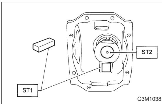
(6) Turn ST1 with hand to make it seated, and tighten drive pinion nut while measuring the preload with spring balance. Select preload adjusting washer and spacer so that the specified preload is obtained when nut is tightened to the specified torque with ST2.
