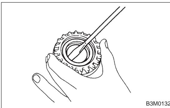
9) Remove oil seal from right and left holders with screwdriver.
