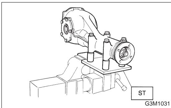
1) Set ST on vise and install the differential assembly to ST.
