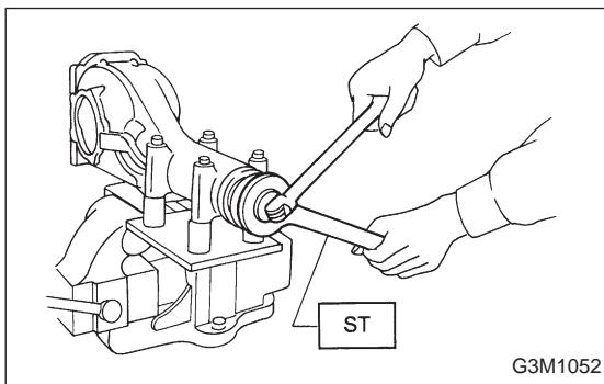
12) Hold companion flange with ST and remove drive pinion nut.
