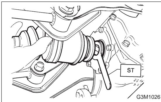
(2) Insert the spline shaft until the spline portion is inside the side oil seal.
