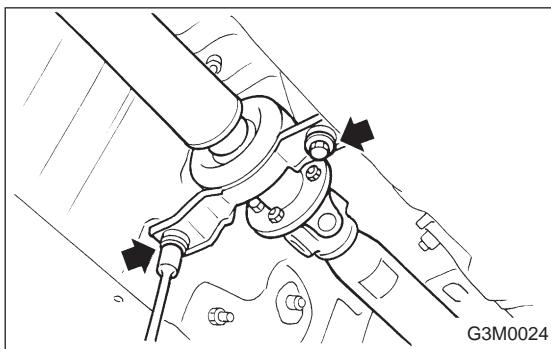
10) Remove propeller shaft.
