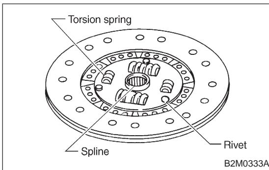
5) Worn spline, loose rivets and torsion spring failure
