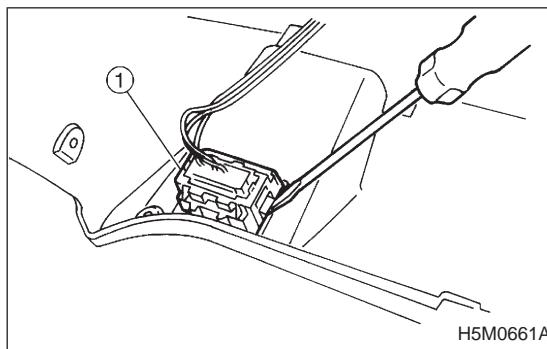
9) Disconnect data link connector ① from lower cover.
