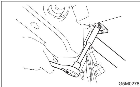
13) Remove two bolts and lower steering column.
