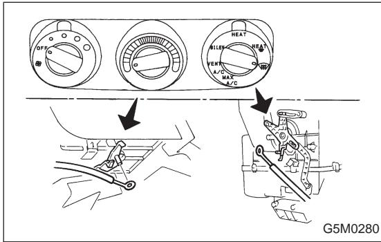
15) Set temperature control switch to Max. COLD, and mode selector switch to defroster position.
