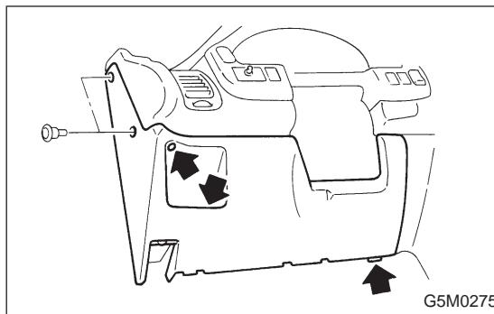
8) Remove lower cover and then disconnect seat belt timer connector.
