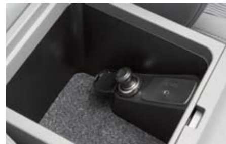
93 Cigarette lighter kit H6710FG000 W Changes the accessory socket to a cigarette lighter.
