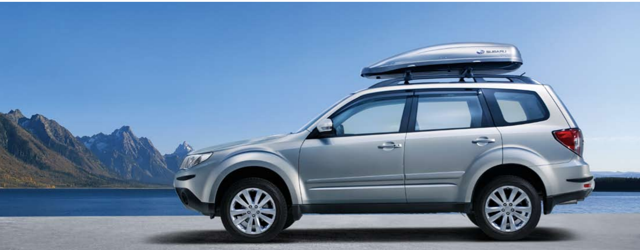
Image: vehicle is presented with Door visors, Side mouldings, Bumper corner protectors, Splash guards, Aluminium carrier base and Transport box (Short).
