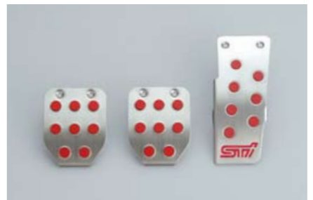
74 STI, Pedal pad set L.H.D. (MT) C8110SA005 Sporty looking set of pedals made of aluminium.
