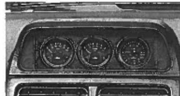
61 Sports gauge pack Oil thermo meter, oil pressure meter and boost meter
