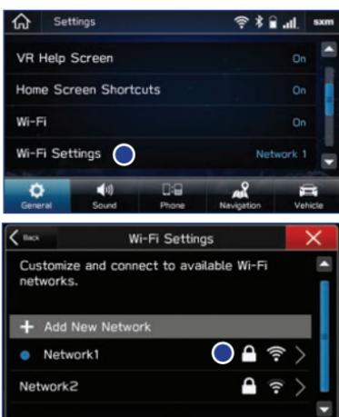
Next, select the desired network. If the network is a secure network, a lock symbol appears on the right side of the screen. Touch the network name and then “Connect” on the next screen. This will take you to a screen to enter the password and then select “Join”.
