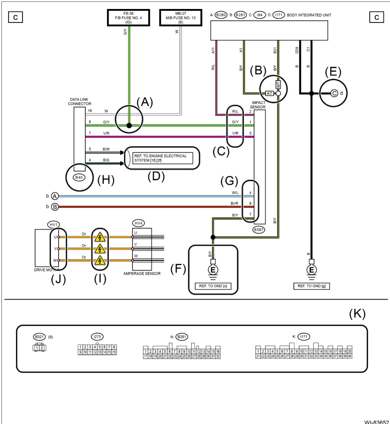
(A) : Wire connection and crossing in a circuit
