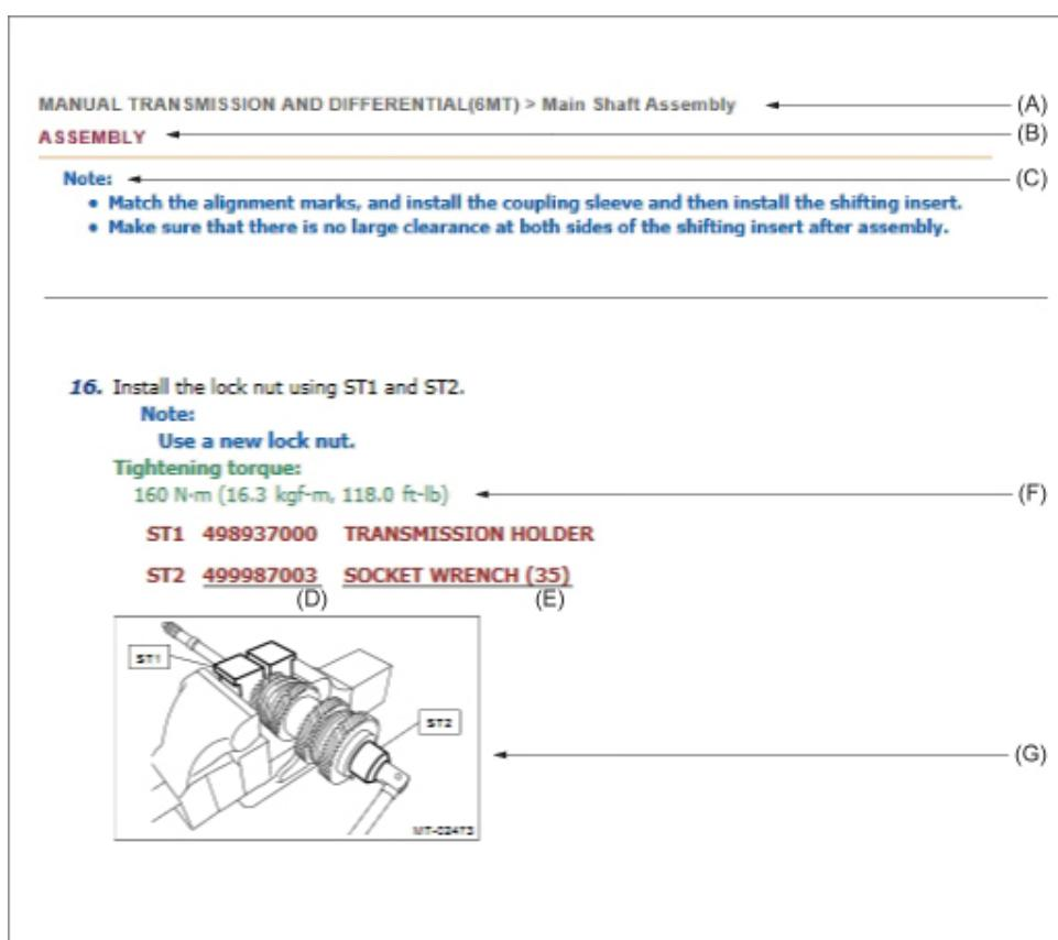
(A) Component (D) Tool number of special tool (F) Tightening torque
