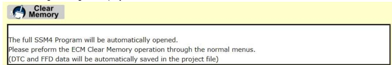
As the SSM4 is automatically started, and displayed on a separate window, the memory clear operation must be carried out using the regular procedure on the SSM4 itself.
