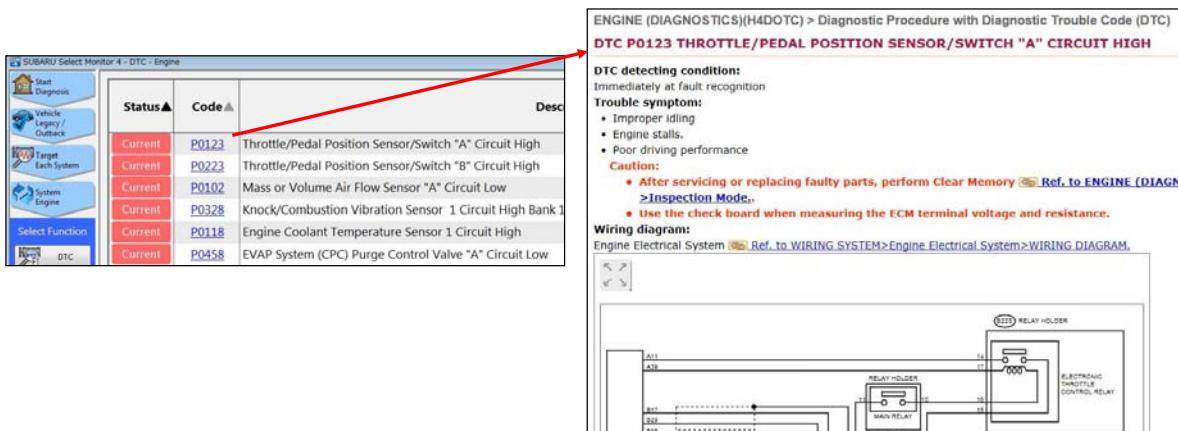
The screenshot shows the SUBARU Select Monitor 4 - DTC - Engine interface. On the left, there is a sidebar with icons for Start Diagnosis, Vehicle Legacy / Outback, Target Test System, System Engine, Select Function, and DTC (which is selected). The main area displays a table of DTCs:
