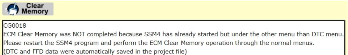
The memory is not able to be automatically cleared when the SSM4 program is running in another window. In this case, the memory clear operation must be carried out using the regular procedure on the SSM4 itself.
