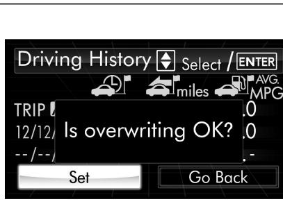
7. To overwrite the previous registration, push the **ENTER** button. When registration is performed the first time, it is registered
