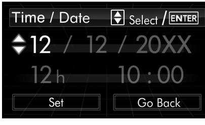
4. Select a number by operating the “▲” or “▼” switch. Then push the **[ENTER]** button. When “12 h” is selected, the clock will be set to a 12-hour display. When “24 h” is selected, the clock will be set to a 24-hour display.
