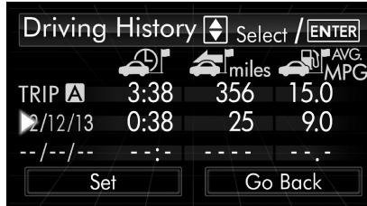
6. Select one of the registration lines by operating the “**▲**” or “**▼**” switch. Then push the **ENTER** button.
