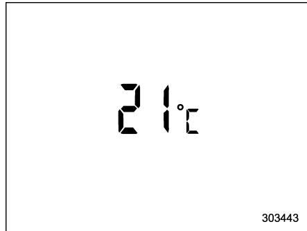
This indicator displays the outside temperature between  $-40^{\circ}\text{F}$  ( $-40^{\circ}\text{C}$ ) and  $122^{\circ}\text{F}$  ( $50^{\circ}\text{C}$ ).
