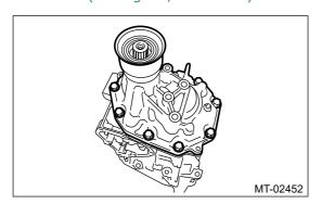
**18.** Temporarily install the gasket to the transmission case side.
