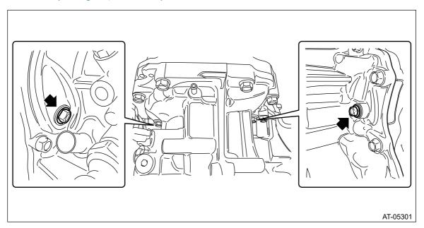
**6.** Set the ST to secondary pulley and expand the V groove of pulley.
