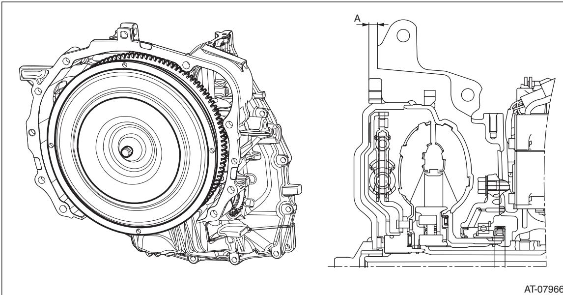
5) Install the transmission assembly to the vehicle. <Ref. to CVT(TR580)-67, INSTALLATION, Automatic Transmission Assembly.>
