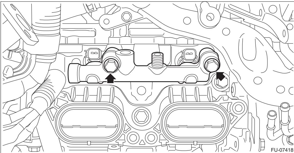
5) Temporarily tighten the fuel pressure sensor to the fuel injector pipe RH until it cannot be turned by hand.
