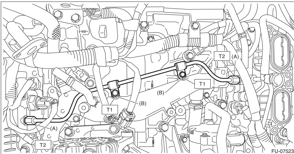
8) Install the fuel pipe insulator No. 3.<Ref. to FU(H4DOTC)-51, FUEL PIPE INSULATOR NO. 3, INSTALLATION, Fuel Insulator.>
