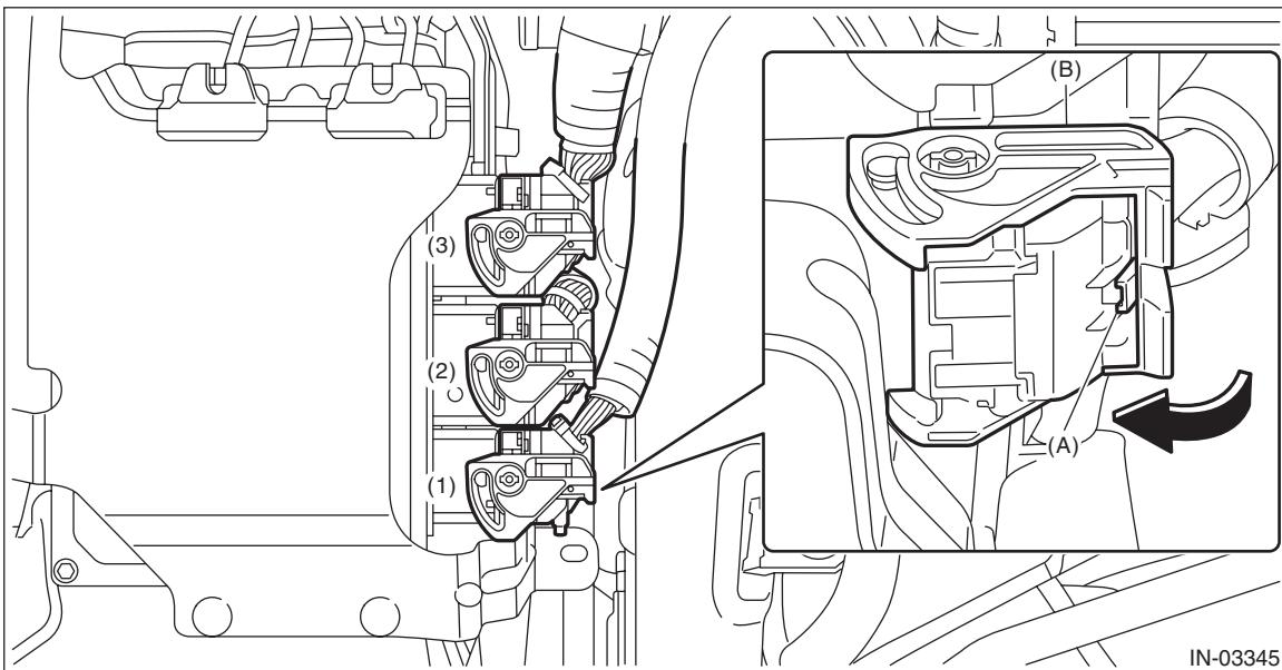
3) Install the special tool between the ECM and body harness and the engine harness. <Ref. to EN(H4DOTC)(diag)-6, CAUTION, General Description.>
