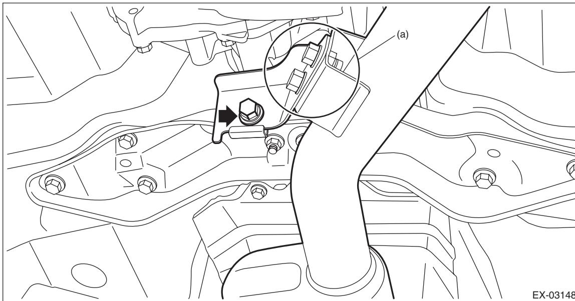
20) Disconnect the union screw pipe assembly from the oil pipe assembly, and disconnect the engine coolant hose (A) from the water pipe RH.
