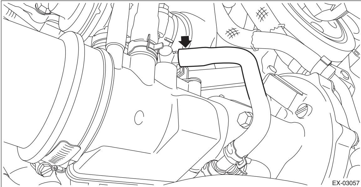
16) Remove the bolts which secure the intake duct No. 1 to the turbocharger.
