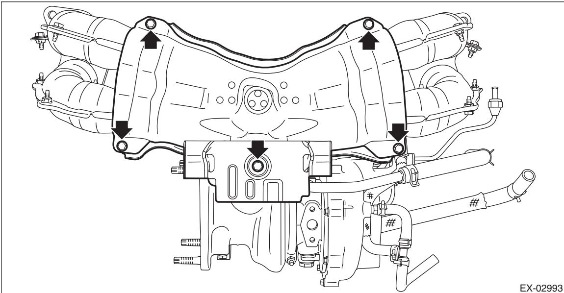
4) Install the center exhaust pipe (front) together with the turbocharger stay (A) to the turbocharger.
