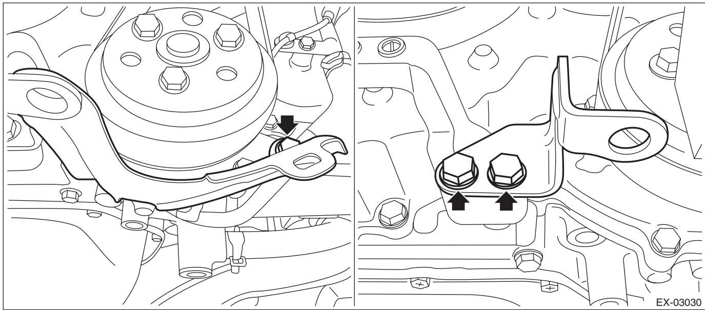
26) Remove the turbocharger stay from the engine.
