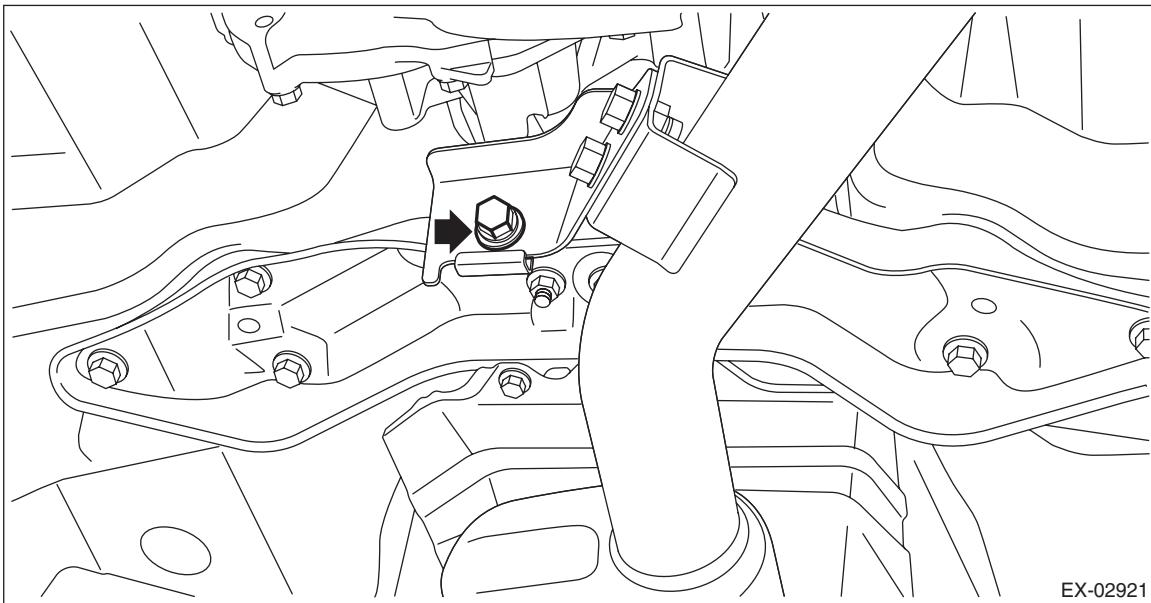
12) Install the bolt which secure the intake duct No. 1 to the turbocharger.
