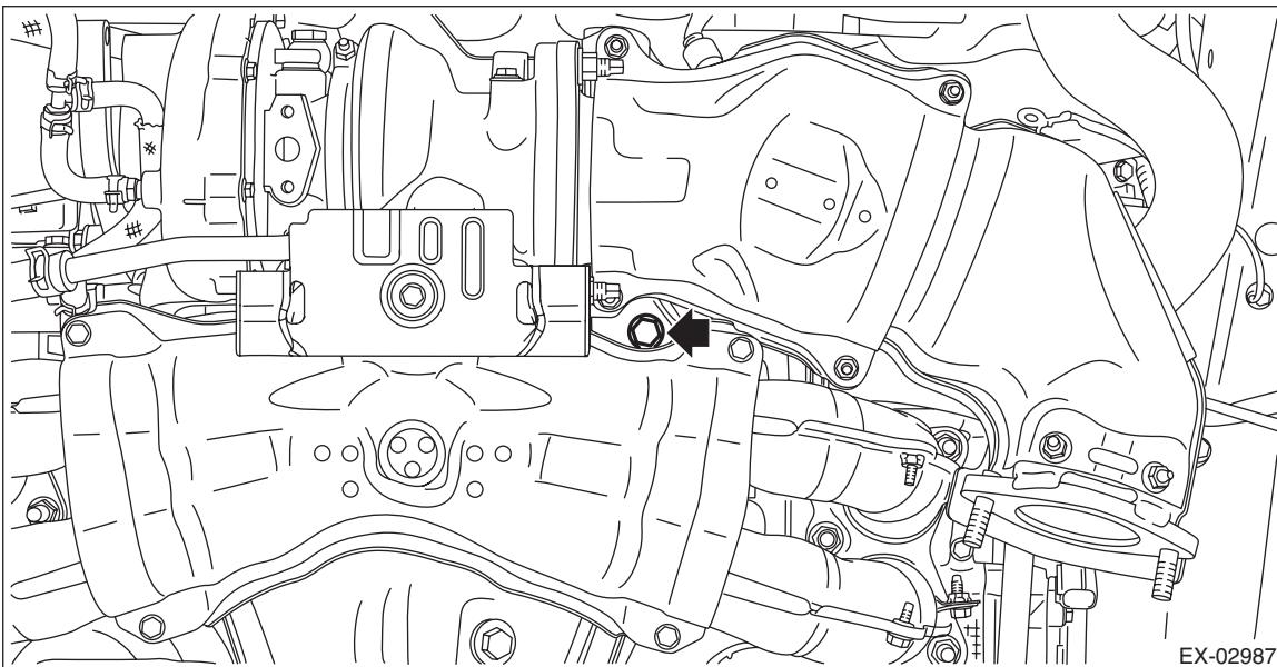
5) Install the oil catch tank to the turbocharger and exhaust stay.
