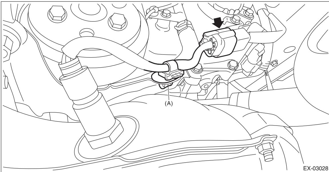
14) Disconnect the connector on the rear oxygen sensor from the engine harness, and disconnect the ground cable from the exhaust pipe cover.
