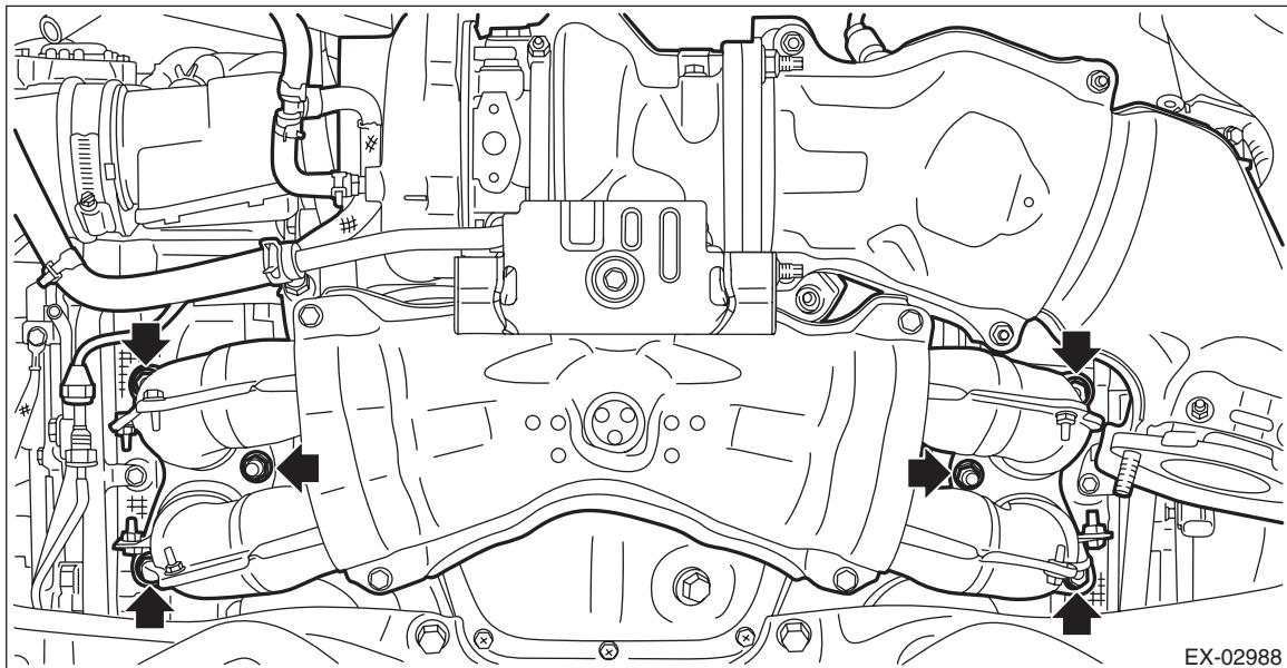
4) Attach the bolt which holds the turbocharger stay.
