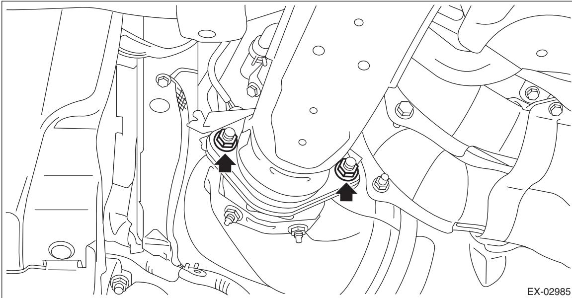
18) Remove the bolts, springs, and nuts which secure the rear exhaust pipe to the center exhaust pipe (rear).
