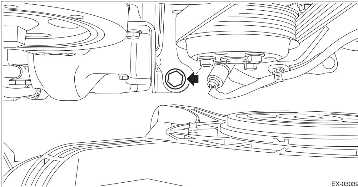
21) Install the radiator sub fan and fan motor assembly. <Ref. to CO(H4DOTC)-56, INSTALLATION, Radiator Sub Fan and Fan Motor.>
