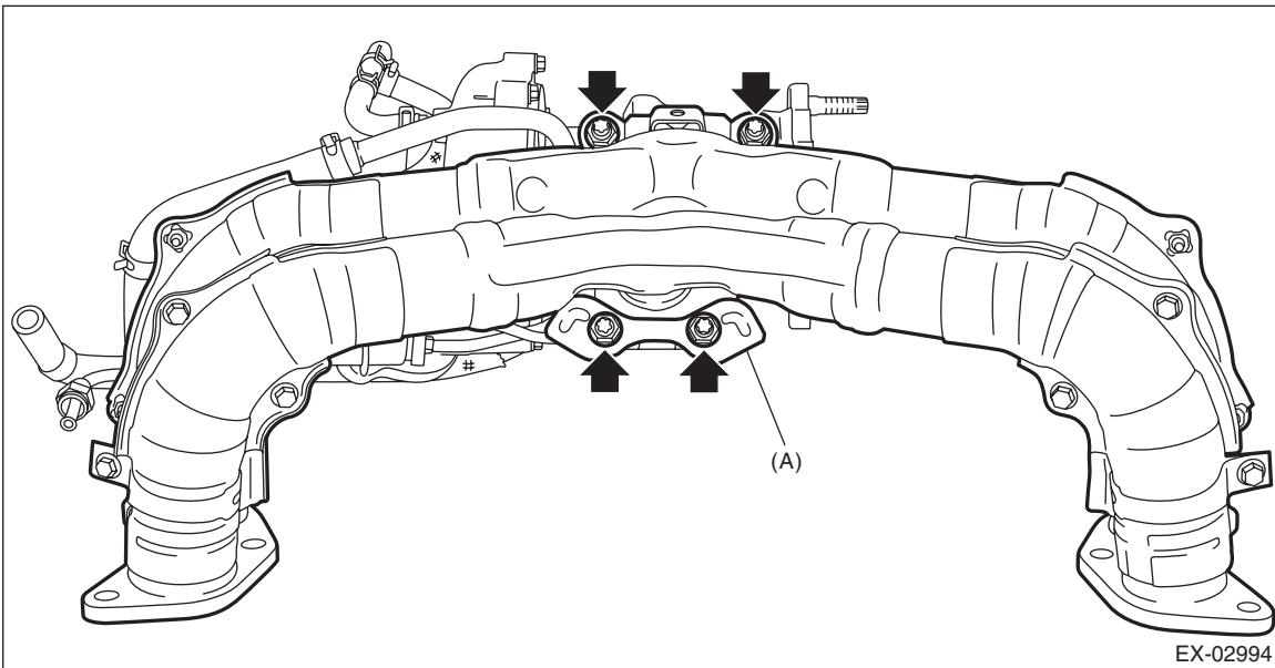
5) Remove the exhaust pipe cover from the front exhaust pipe.
