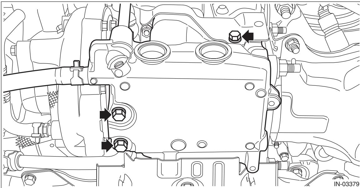
23) Remove the bolts which secure the turbocharger stay.
