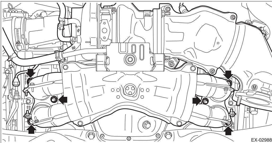
25) Remove the water pump pulley cover and exhaust pipe stay from the engine and turbocharger stay.
