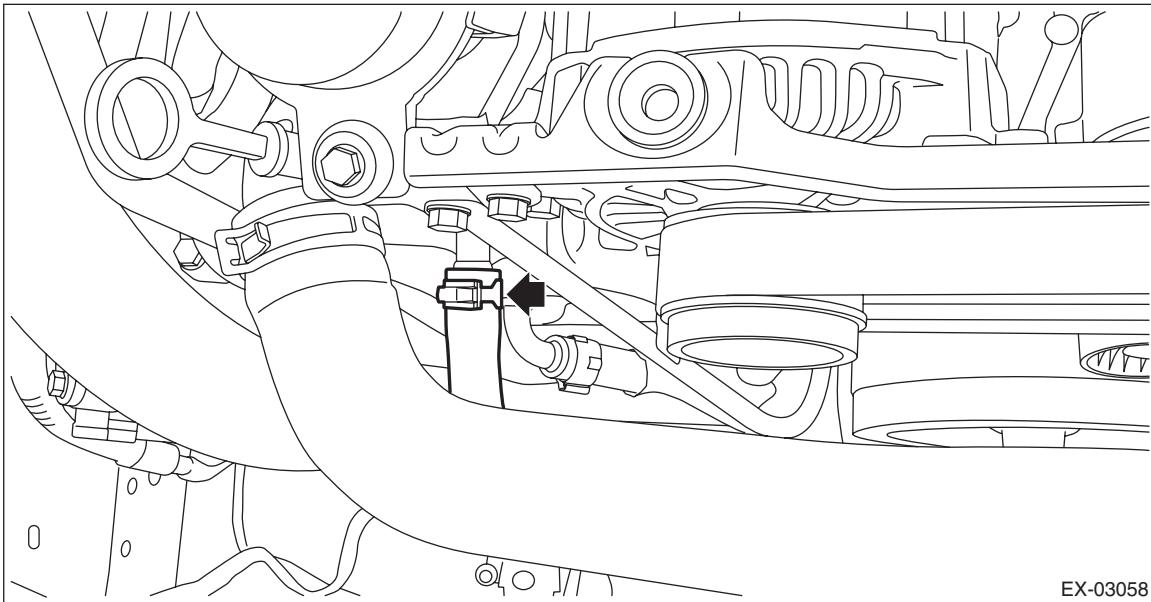
11) Remove the bolts which secure the intake duct No. 2 to the turbocharger.
