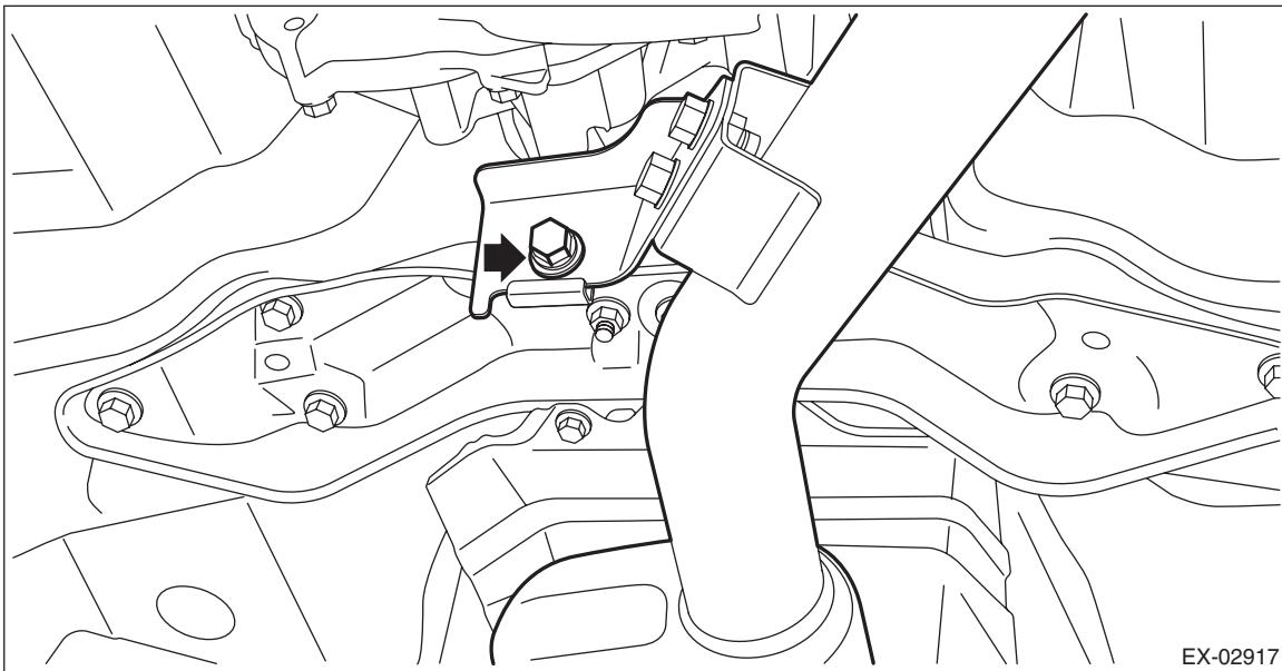
9) Install the bolts, springs, and nuts which secure the rear exhaust pipe to the center exhaust pipe (rear).
