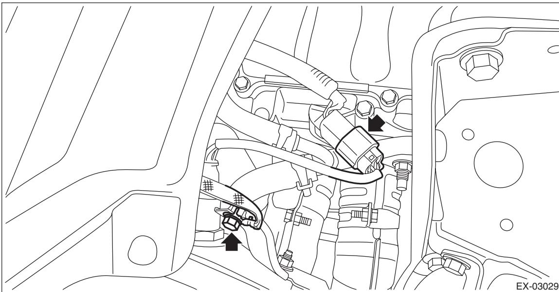
15) Secure the front oxygen (A/F) sensor harness to the water pump pulley cover with the clip (A), and connect the front oxygen (A/F) sensor connector to the engine harness.
