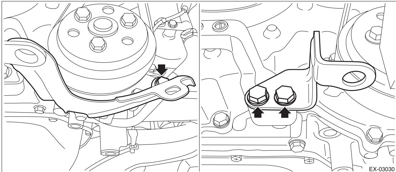
3) While holding the front exhaust pipe with transmission jack, set the front exhaust pipe, and install the nuts which hold the front exhaust pipe to the cylinder head exhaust port.
