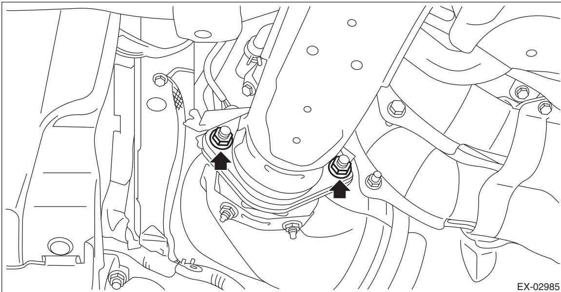
11) Tighten the bolts which hold center exhaust pipe (rear) to the hanger bracket.
