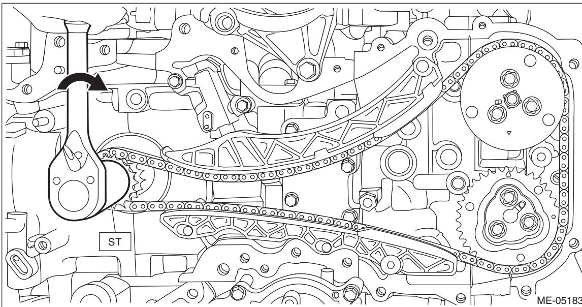
11) Using ST and by turning the crankshaft, align the alignment marks of crank sprocket, intake cam sprocket LH and exhaust cam sprocket LH to the positions as shown in the figure.
