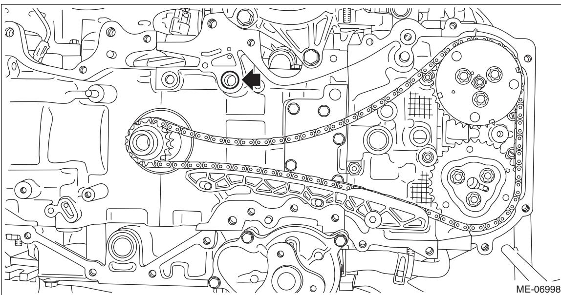
6) Remove the chain guide LH, and remove the timing chain LH (A).
