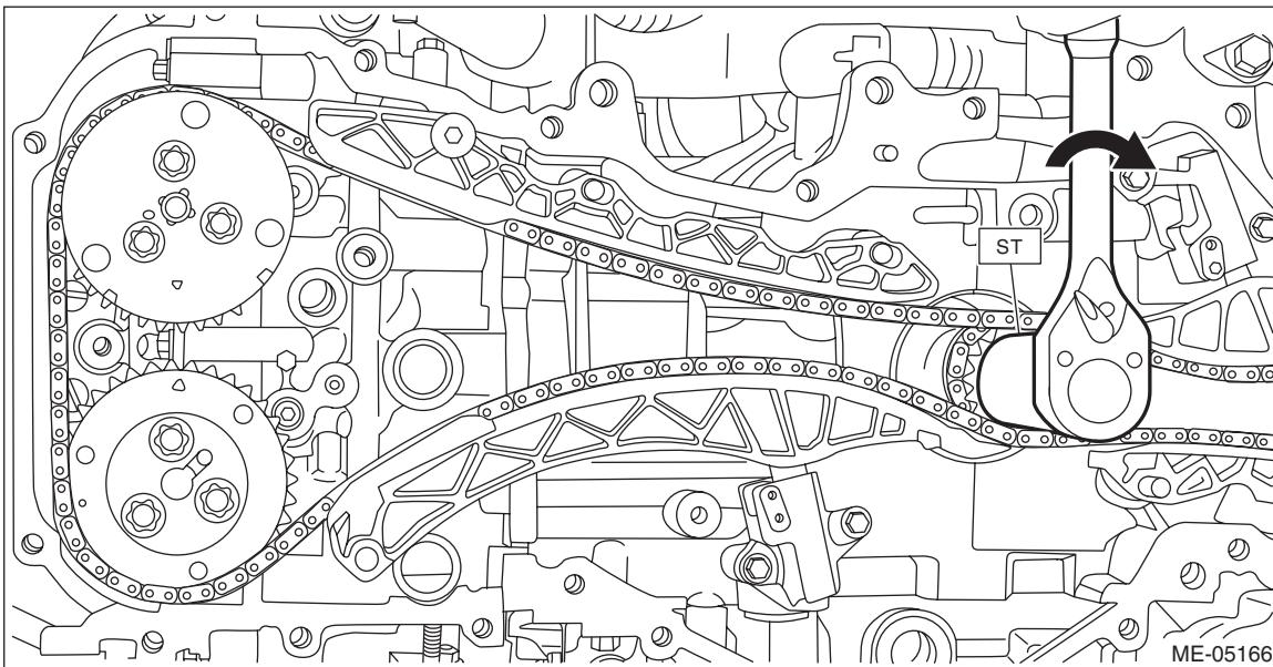
10) Install the chain cover. <Ref. to ME(H4DO)-111, INSTALLATION, Chain Cover.>
