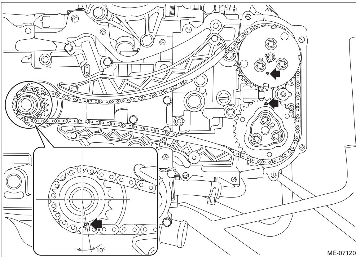
4) Align the alignment marks of intake cam sprocket RH and exhaust cam sprocket RH to the positions as shown in the figure.
