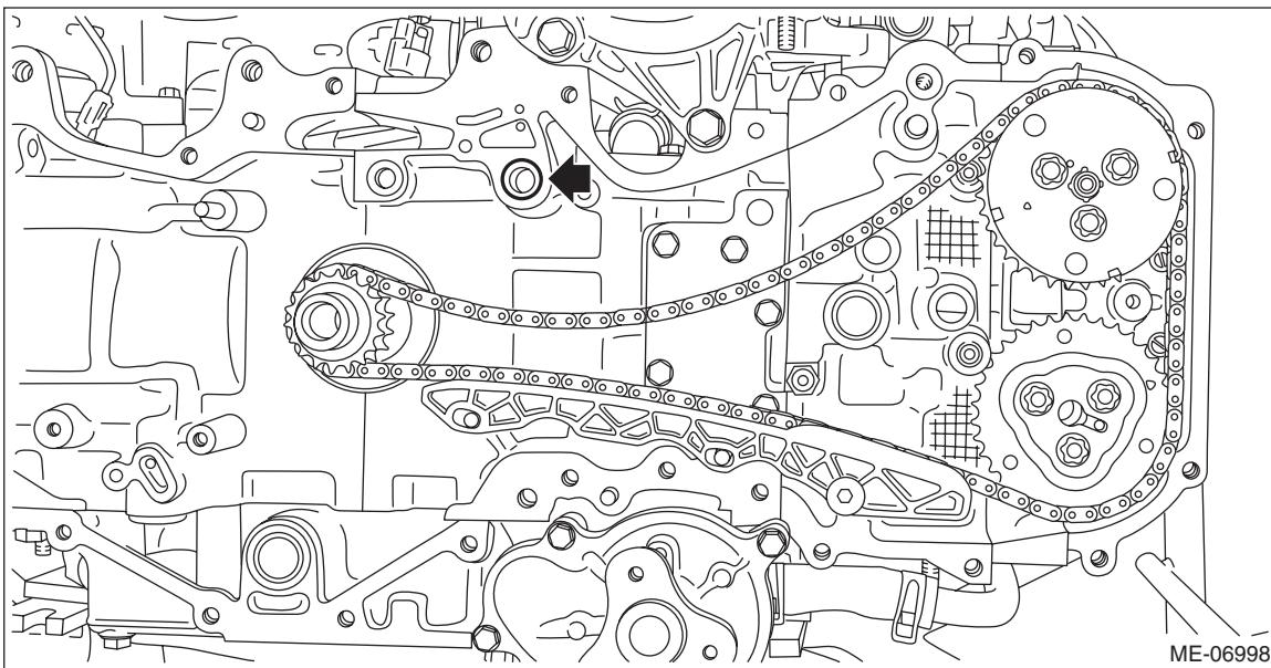
8) Install the chain tensioner lever LH (A) and chain tensioner LH.
