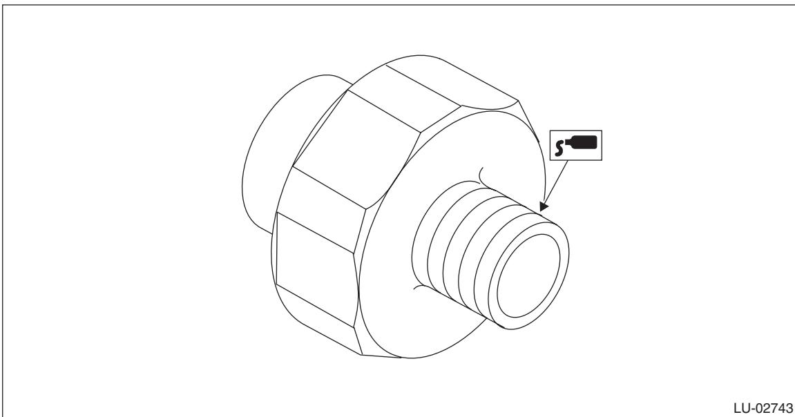
2) Install the oil pressure switch to the chain cover.
