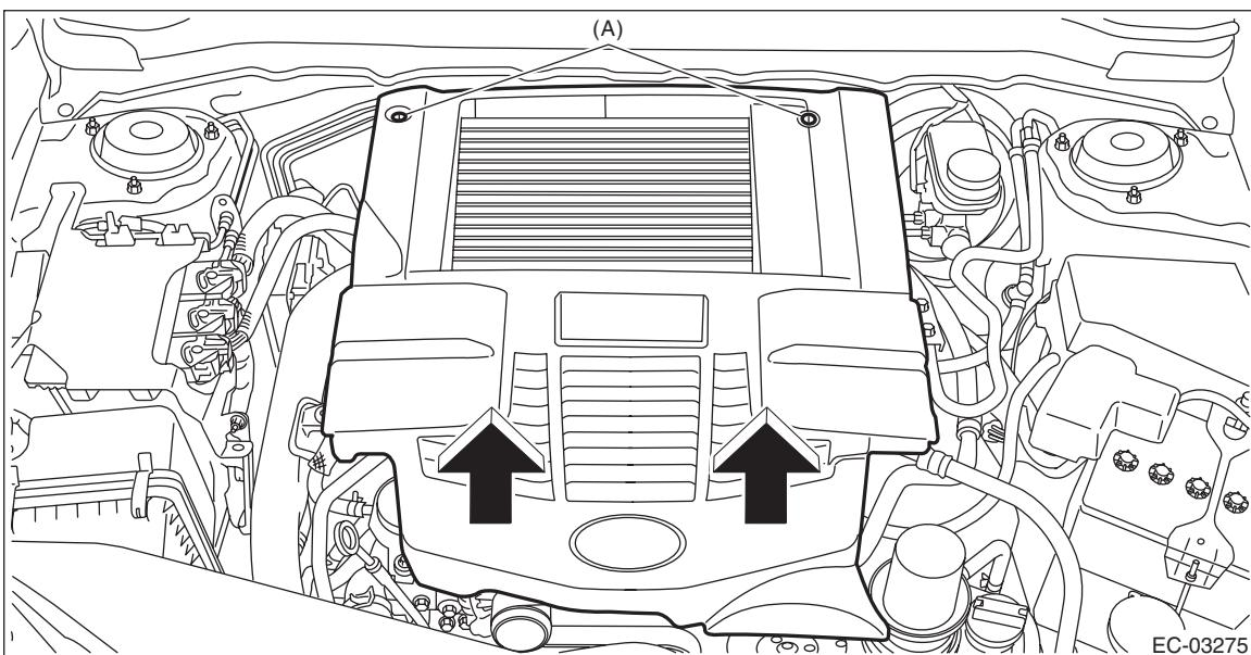
2) Remove the intake duct No. 2. <Ref. to IN(H4DOTC)-22, INTAKE DUCT NO. 2, REMOVAL, Intake Duct.>
