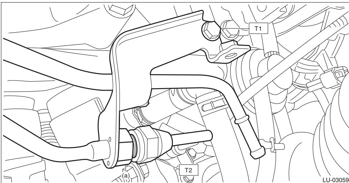
6) Connect the oil outlet hose (B) to the oil pipe assembly, and install the ground cable (A) to the oil pipe assembly.
