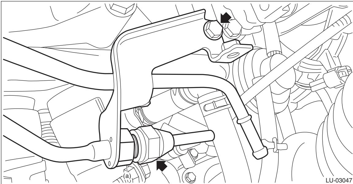
9) Remove the bolt which secures the oil pipe assembly to the cam carrier RH.
