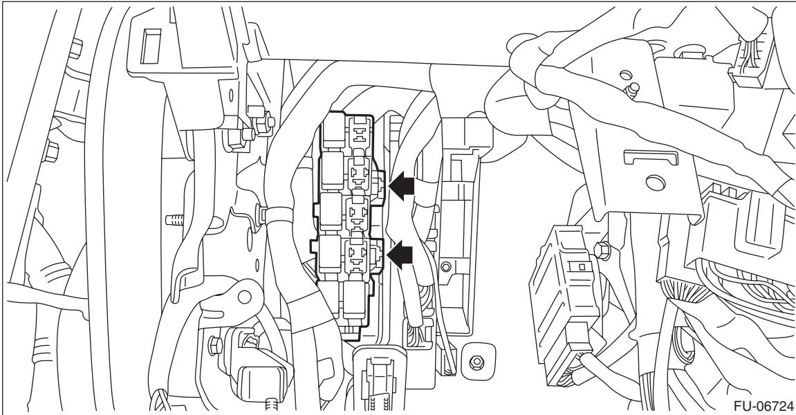
(6) Disconnect the connector from body integrated unit.
