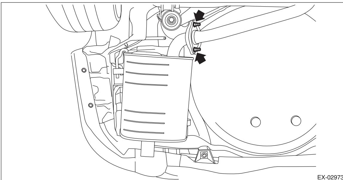
4) Install the bolts, springs, and nuts which secure the center exhaust pipe to the rear exhaust pipe.
