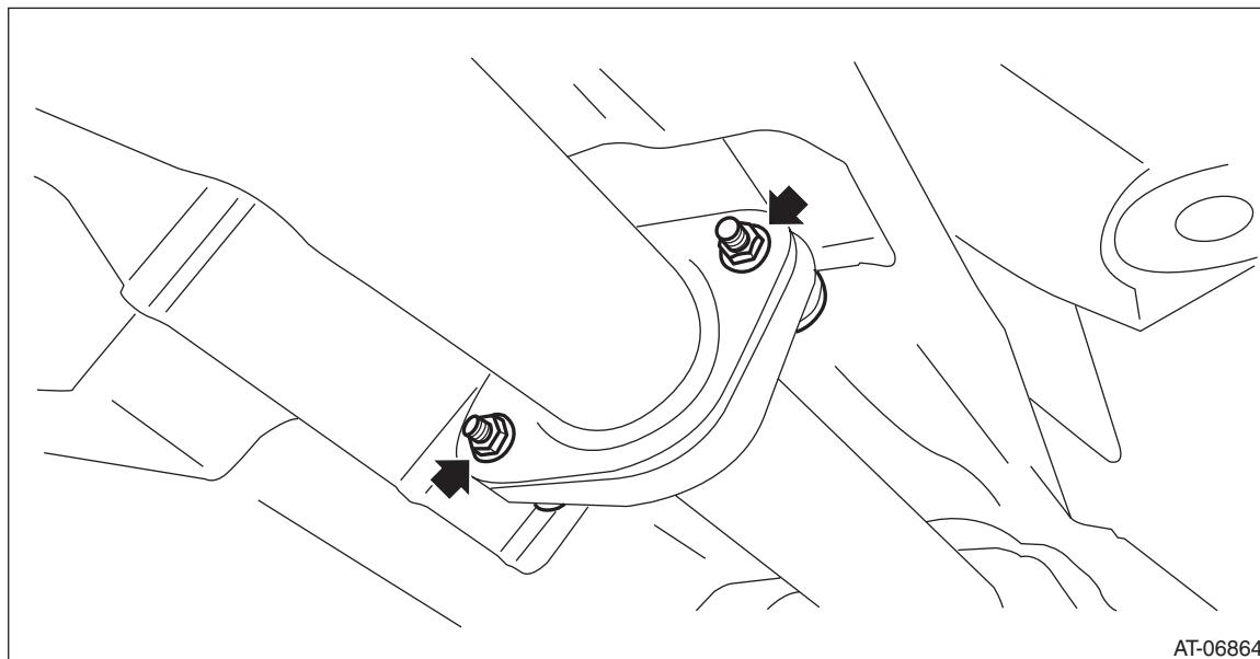
3) Remove the bolts and self-locking nuts securing the mufflers to the rear exhaust pipes.
