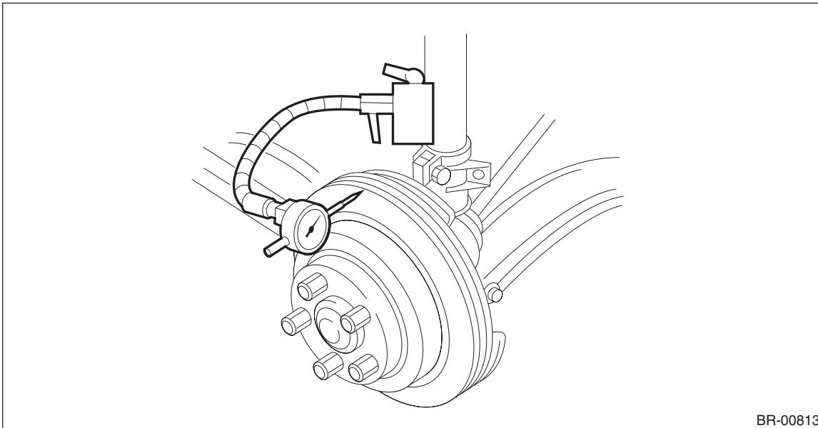
4) If the runout limit is exceeded in the inspection, replace the disc rotor.
