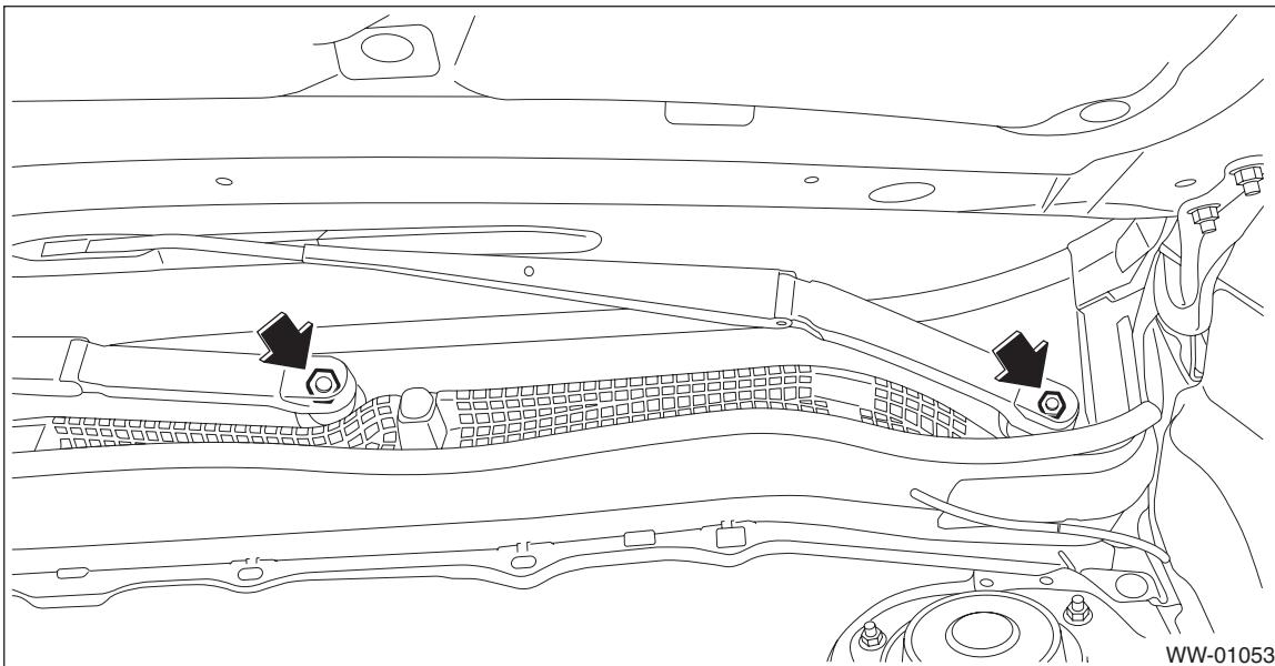
2) Check the position of windshield wiper.<Ref. to WW-28, ADJUSTMENT, Front Wiper Arm.>
