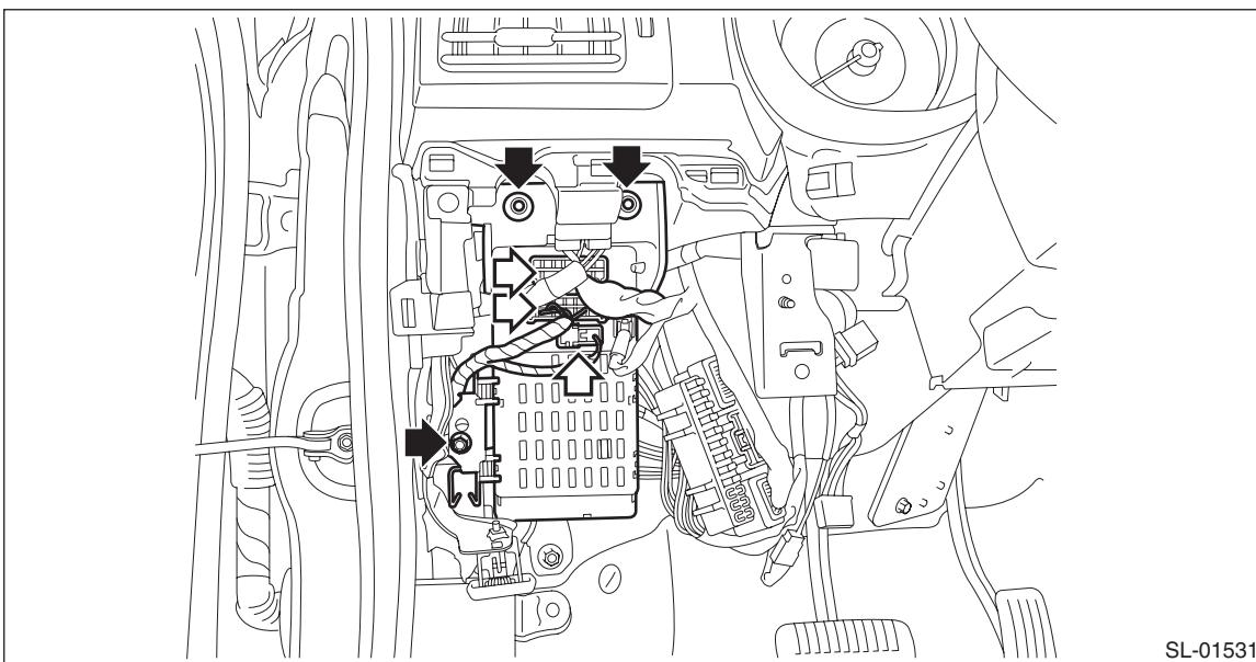
4) Remove the starter cut relay (A) from the relay holder.
