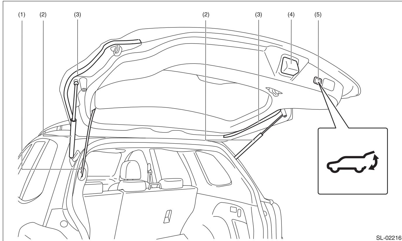
(1) Rod - power rear gate (3) Power rear gate touch sensor (5) Power rear gate inner switch
