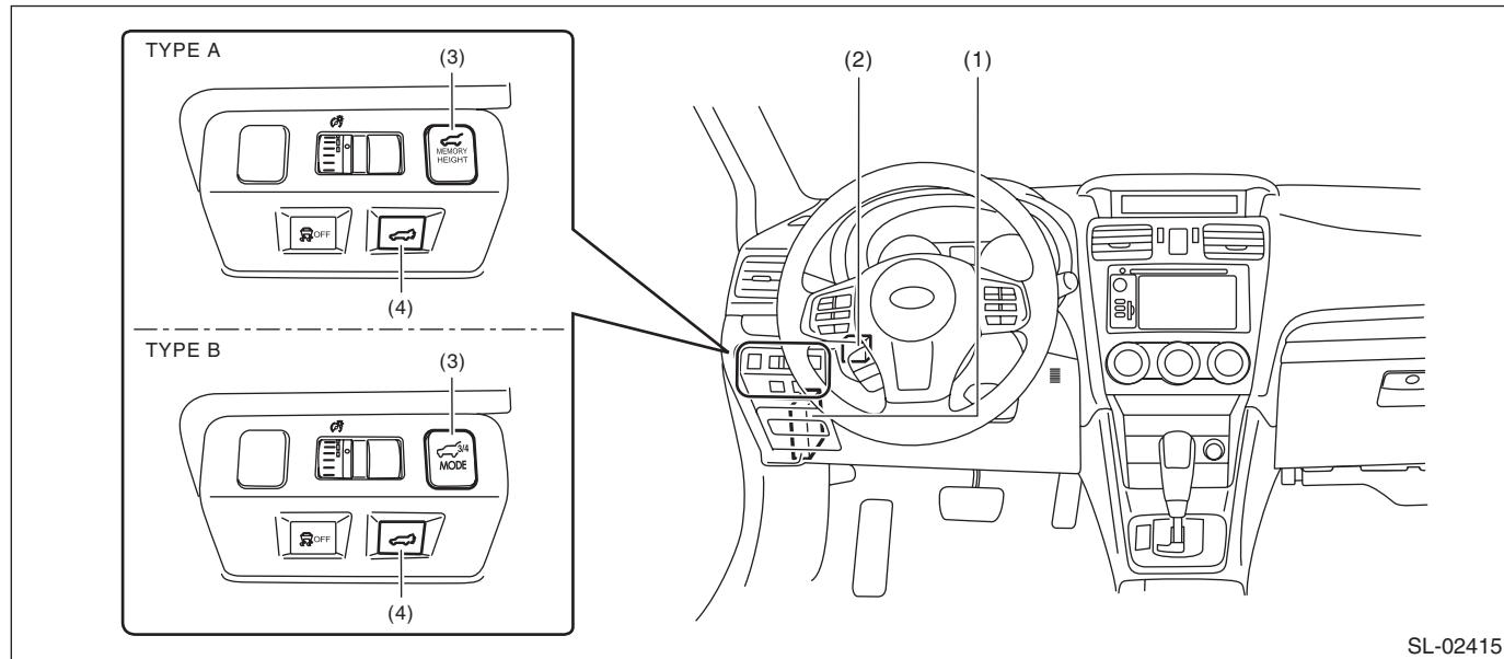
(1) Body integrated unit (3) Memory height switch (4) Power rear gate driver's switch
