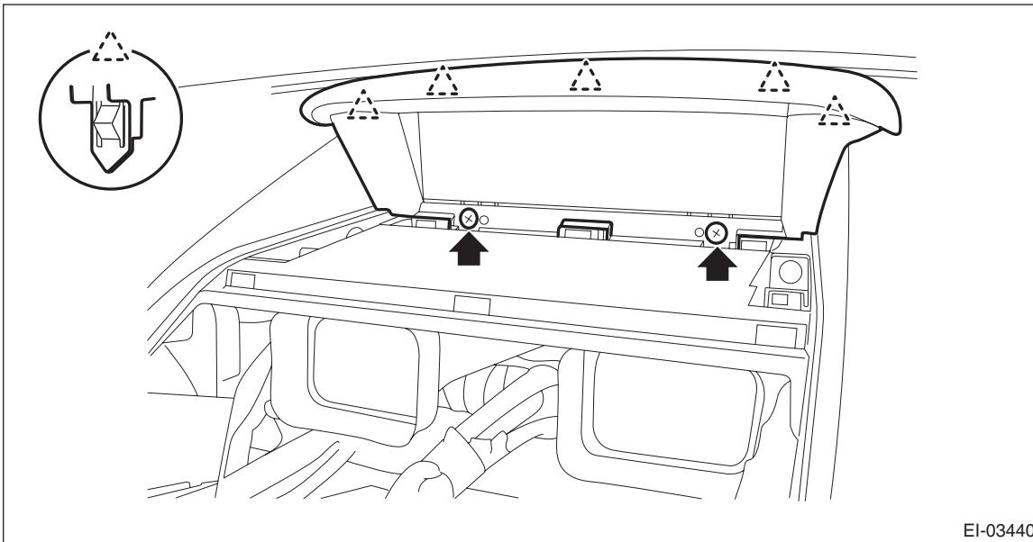
(3) Remove the screw, and remove the multi-function display from the panel - display.
