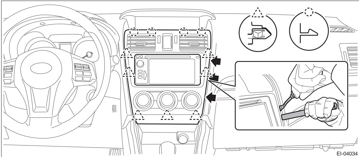
3) Release the claws, and then remove the grille assembly - CTR ventilation from the panel center assembly.
