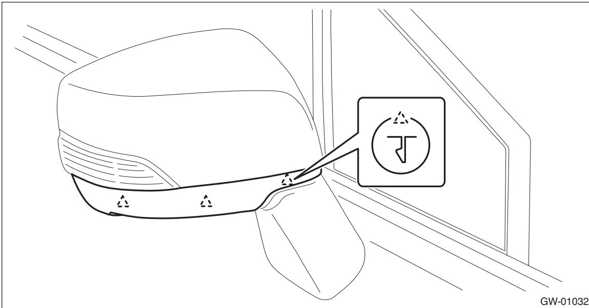
5) Release the claws, and then remove the cover - cap outer mirror.
