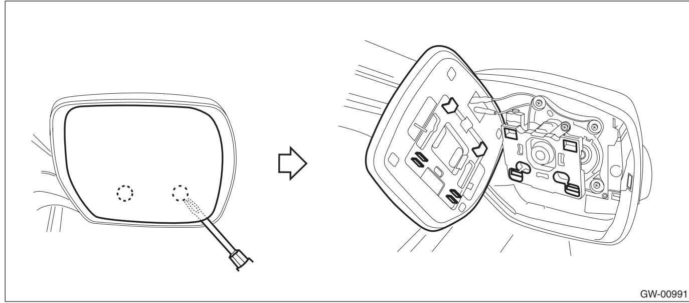
(2) Disconnect the mirror heater connector. (Model with mirror heater)
