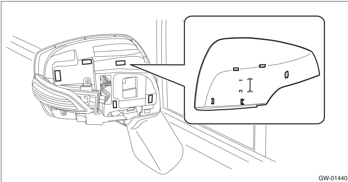
3) Engage the claws into the hole and install the cover - cap outer mirror lower.
