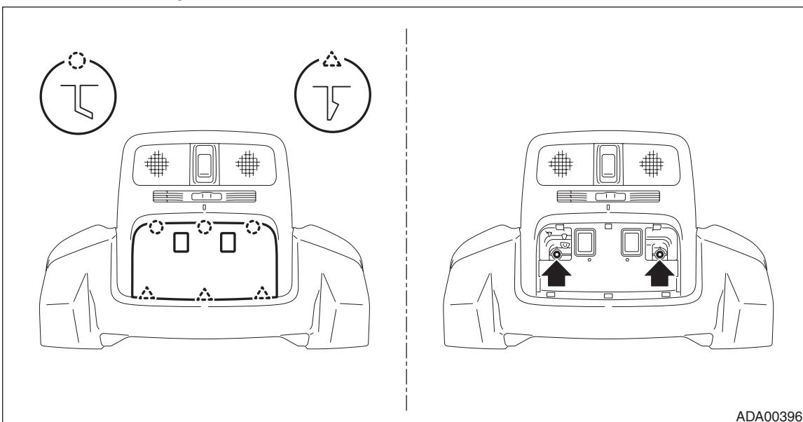
(3) Pull down the rear of the stereo camera cover, and then release the clips.
