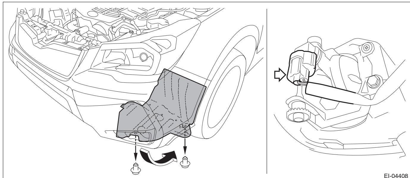
(2) Remove the clips at the upper side of the bumper face - front.
