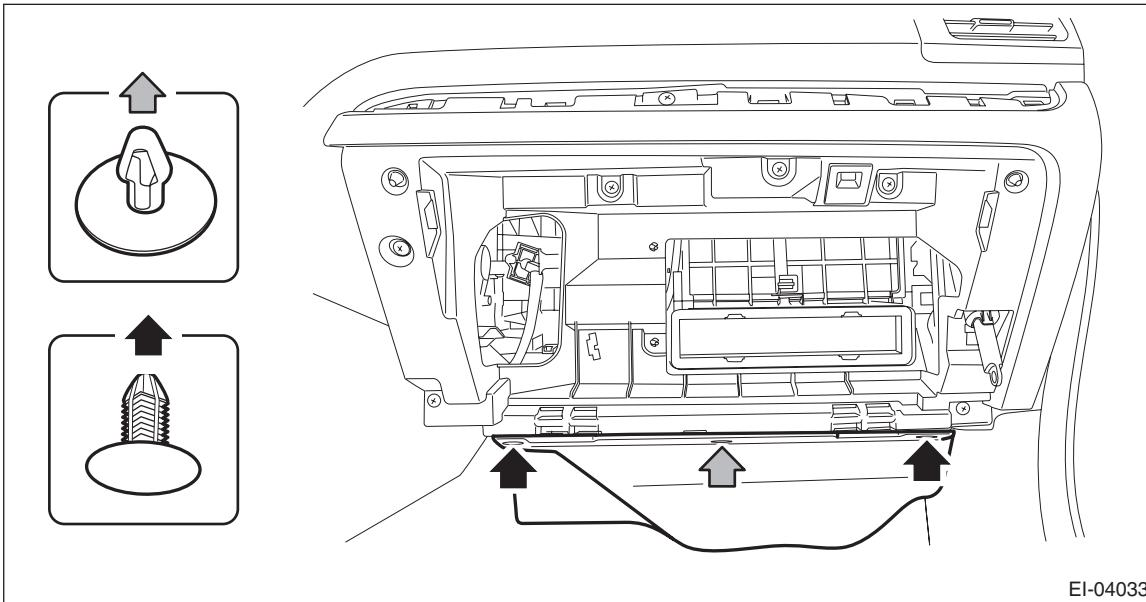
(4) Remove the screws, claws and harness clamp, then remove the back panel - pocket.
