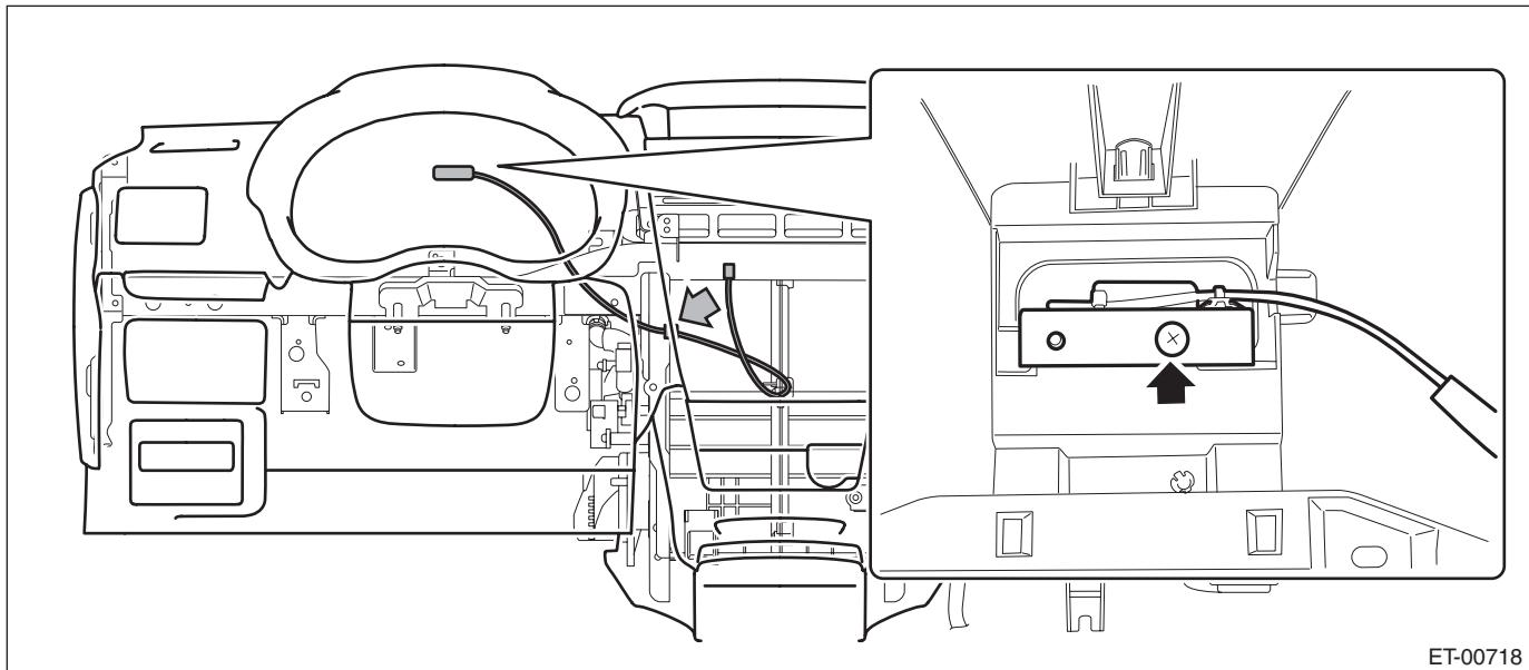
(3) When the GPS antenna assembly is pulled out, remove the string attached to the connector in step (1).
