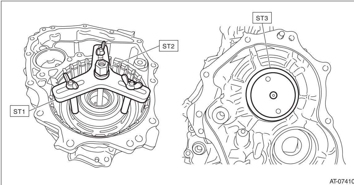
4) Compress the return spring using the set ST to remove the snap ring.
