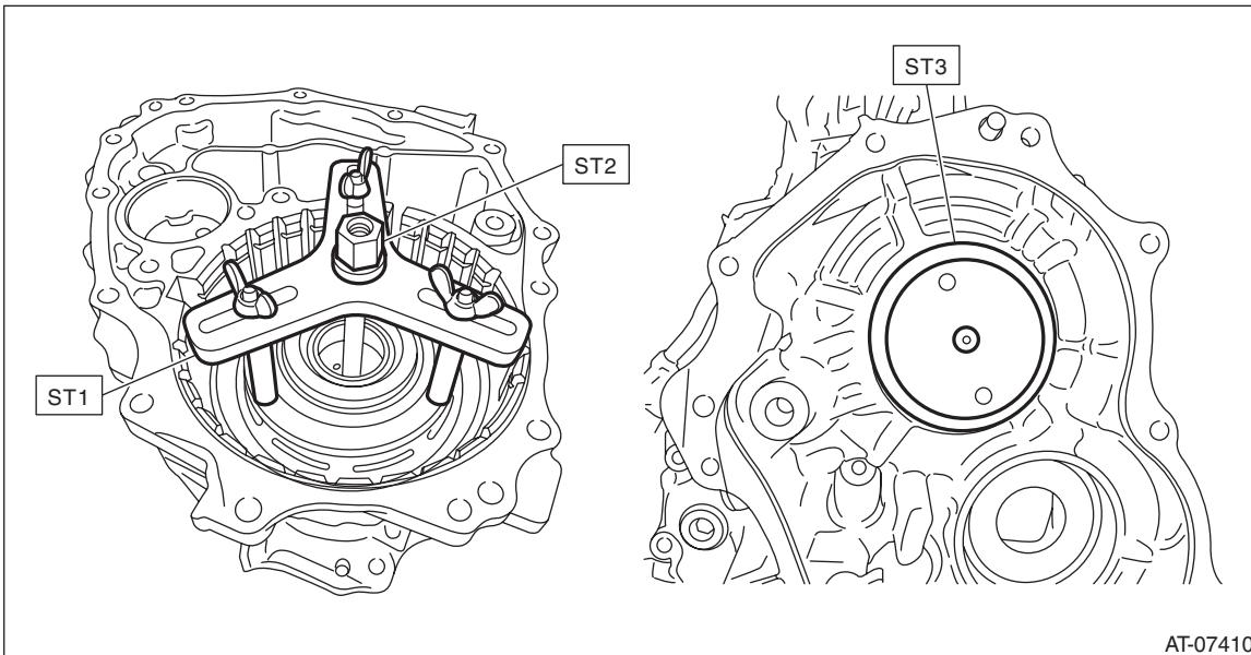
5) Compress the return spring using the ST attached, and install the snap ring.
