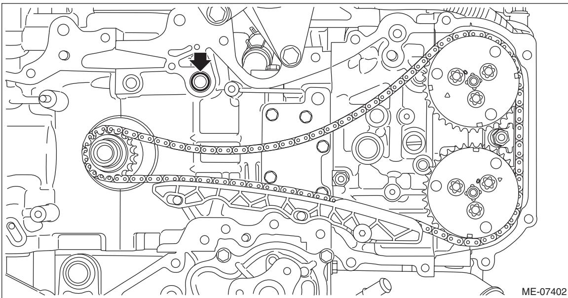
9) Install the chain tensioner lever LH (A) and chain tensioner LH.
