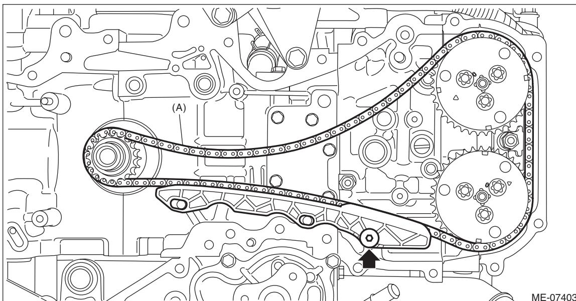
7) Using ST and by turning the crankshaft approximately 200° clockwise, align the alignment marks of crank sprocket to the positions as shown in the figure.
