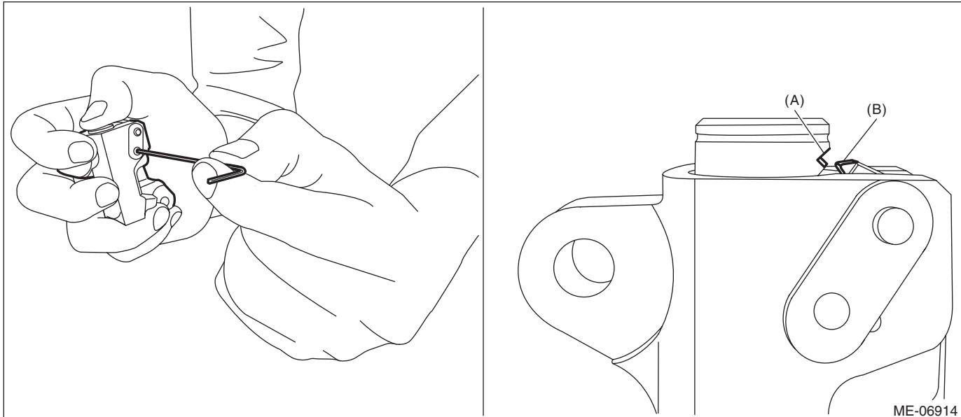
3) Check that the crank sprocket is located at the position shown in the figure. If not aligned, using ST turn the crankshaft to align the crank sprocket alignment mark to the position shown in the figure.
