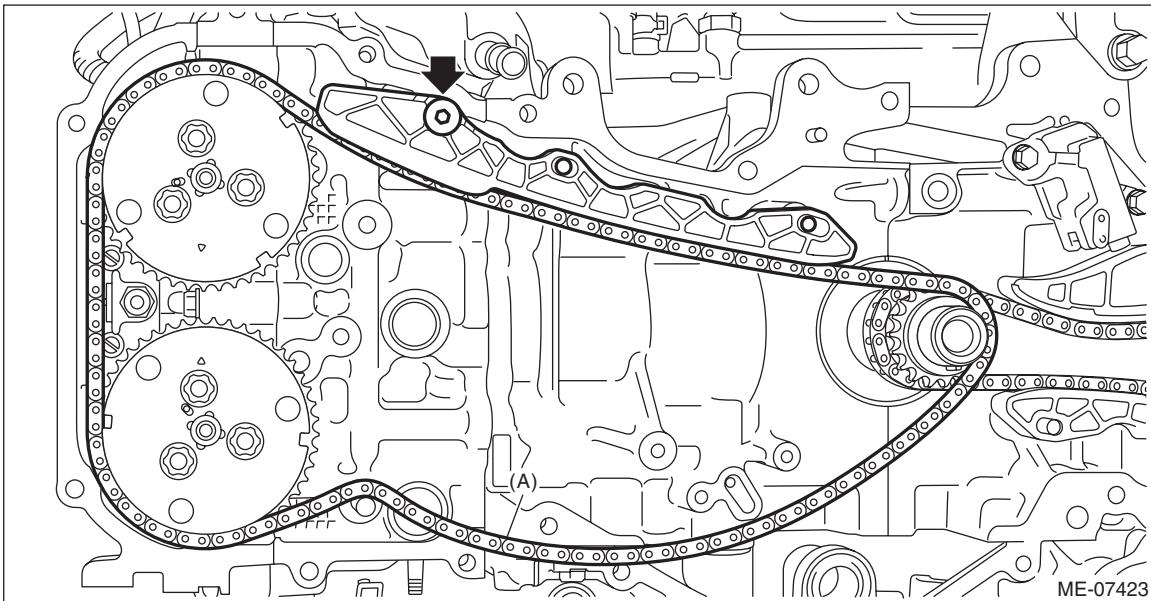
6) Remove the chain guide RH from the front camshaft cap RH.
