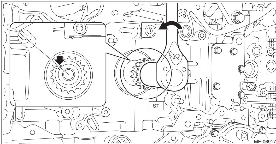
6) Align the alignment mark of exhaust cam sprocket LH to the position shown in the figure.
