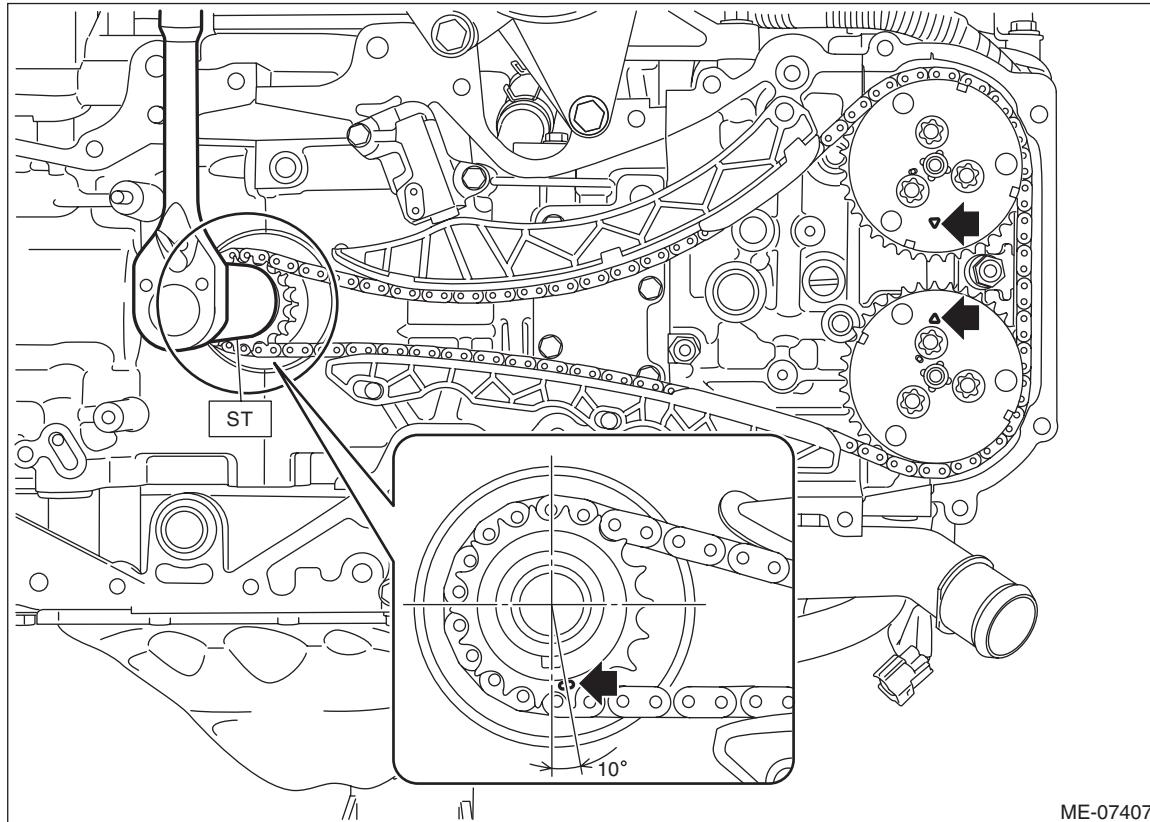
13) Install the timing chain RH. <Ref. to ME(H4DOTC)-129, TIMING CHAIN RH, INSTALLATION, Timing Chain Assembly.>
