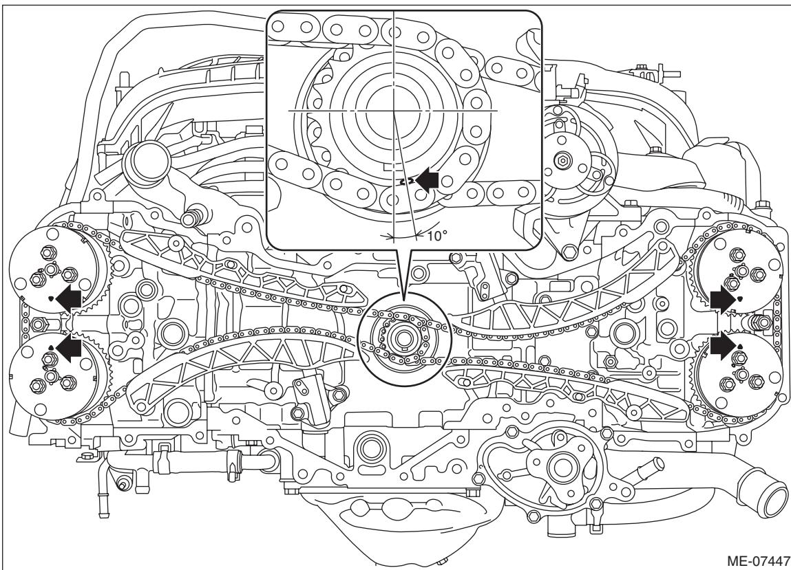
10) Using the ST, turn the crankshaft clockwise, and make sure that there are no abnormal conditions.
