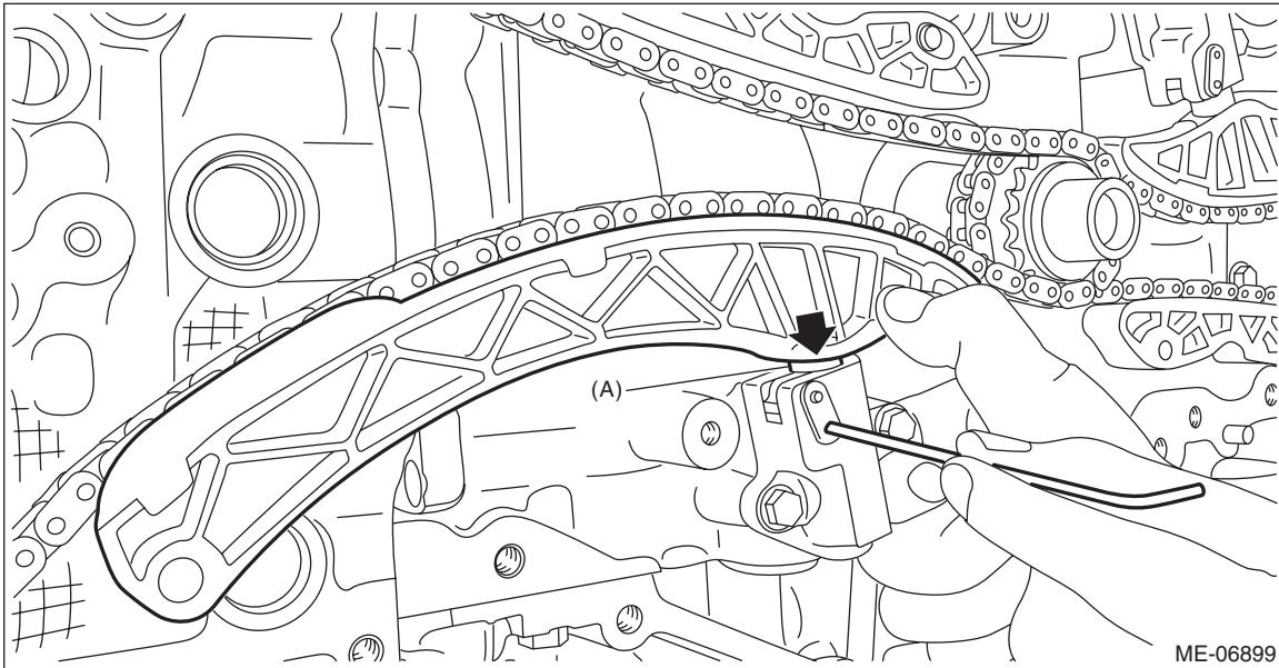
4) Remove the chain tensioner RH, and remove the chain tensioner lever RH (A).
