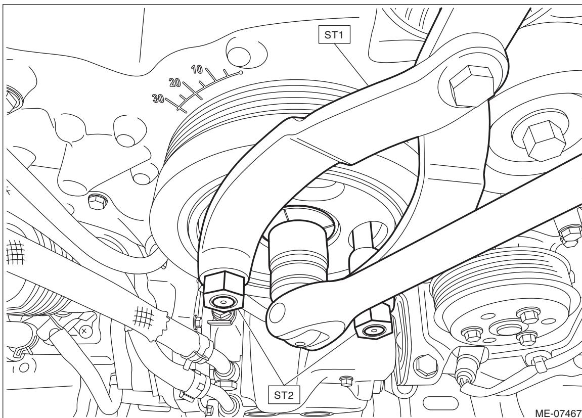
4) Remove the crank pulley.
