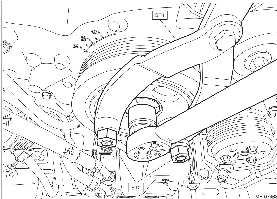
(3) Use the marker as shown in the figure, draw the reference line (A) on the crank pulley bolt according to the indented line on the crank pulley bolt head, and draw the end line (B) on the crank pulley.
