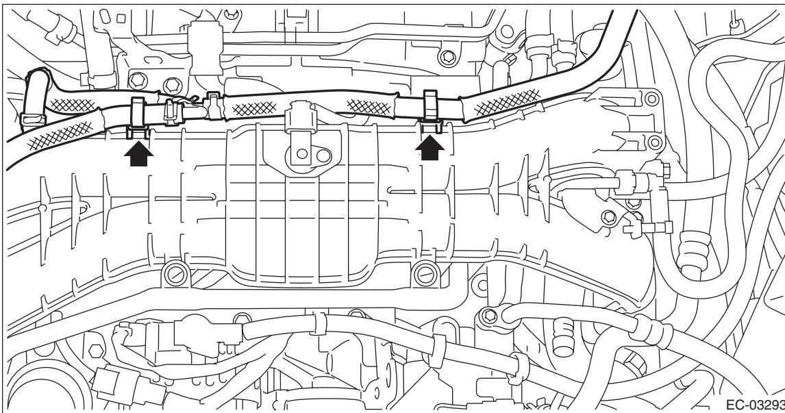
3) Install the intercooler. <Ref. to IN(H4DOTC)-37, INSTALLATION, Intercooler.>
