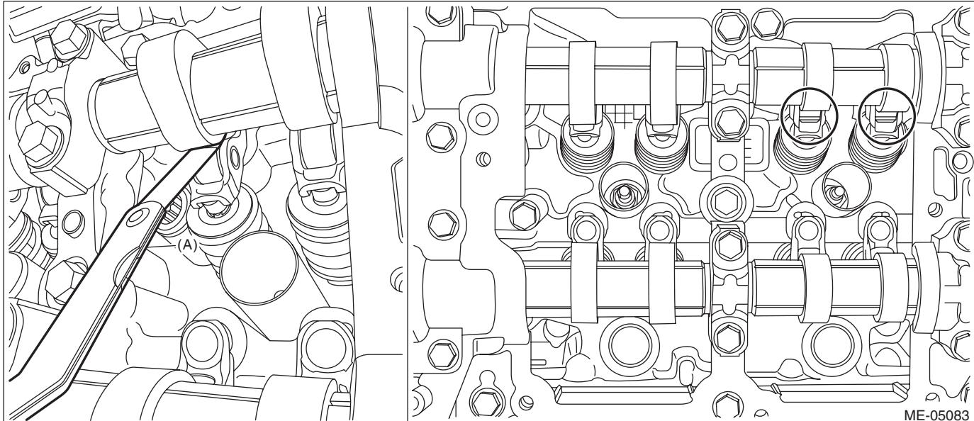
5) If necessary, adjust the cam clearance. <Ref. to ME(H4DO)-47, ADJUSTMENT, Cam Clearance.>
