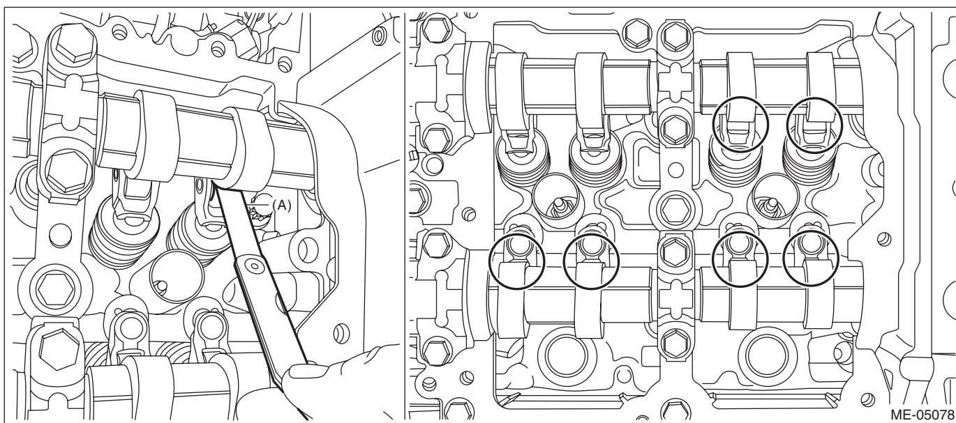
(4) Turn the crank pulley by 360°.
