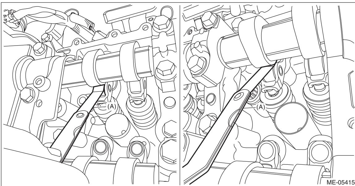
3) If necessary, adjust the cam clearance. <Ref. to ME(H4DO)-47, ADJUSTMENT, Cam Clearance.>
