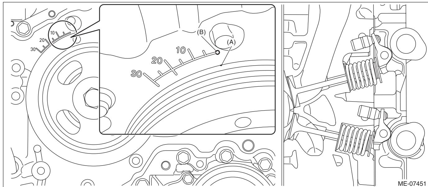
(3) Check the cam clearance for #2 cylinder intake, #2 cylinder exhaust and #4 cylinder exhaust.
