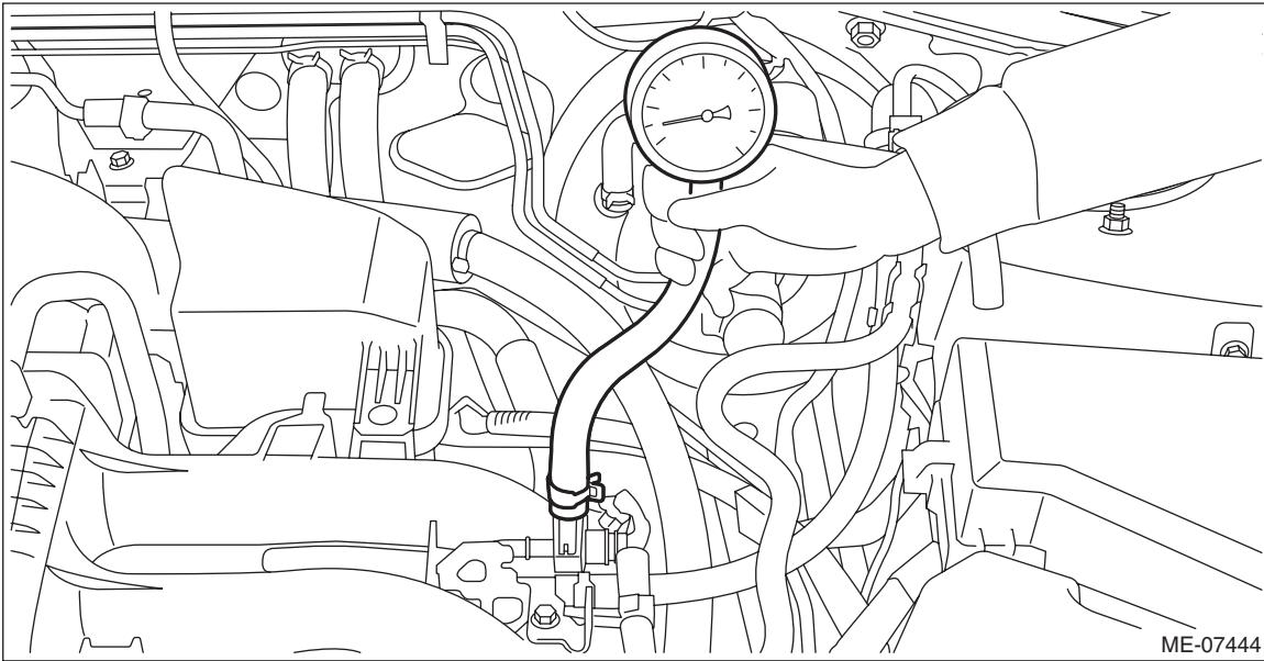
4) Keep the engine at idle speed and read the vacuum gauge indication.
