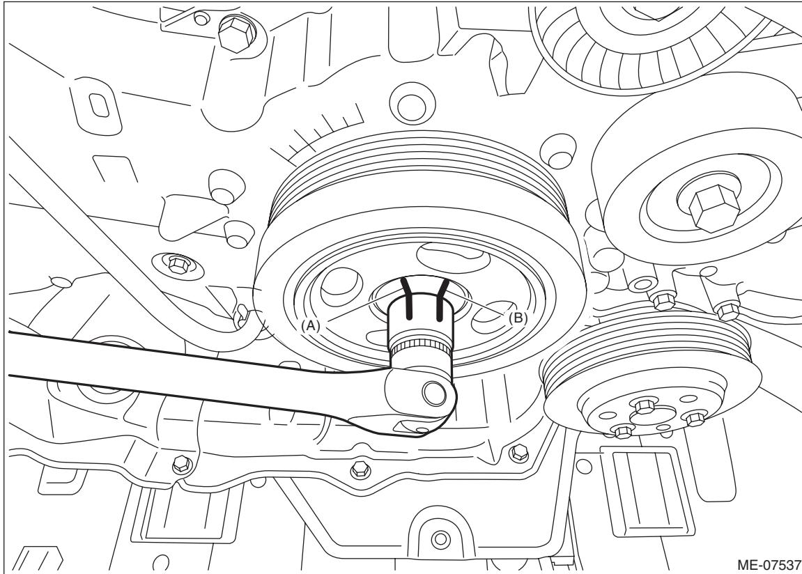
(5) Draw end line (C) on crank pulley using a marker at the same position as reference line (B) drawn on the crank pulley bolt in step (4).
