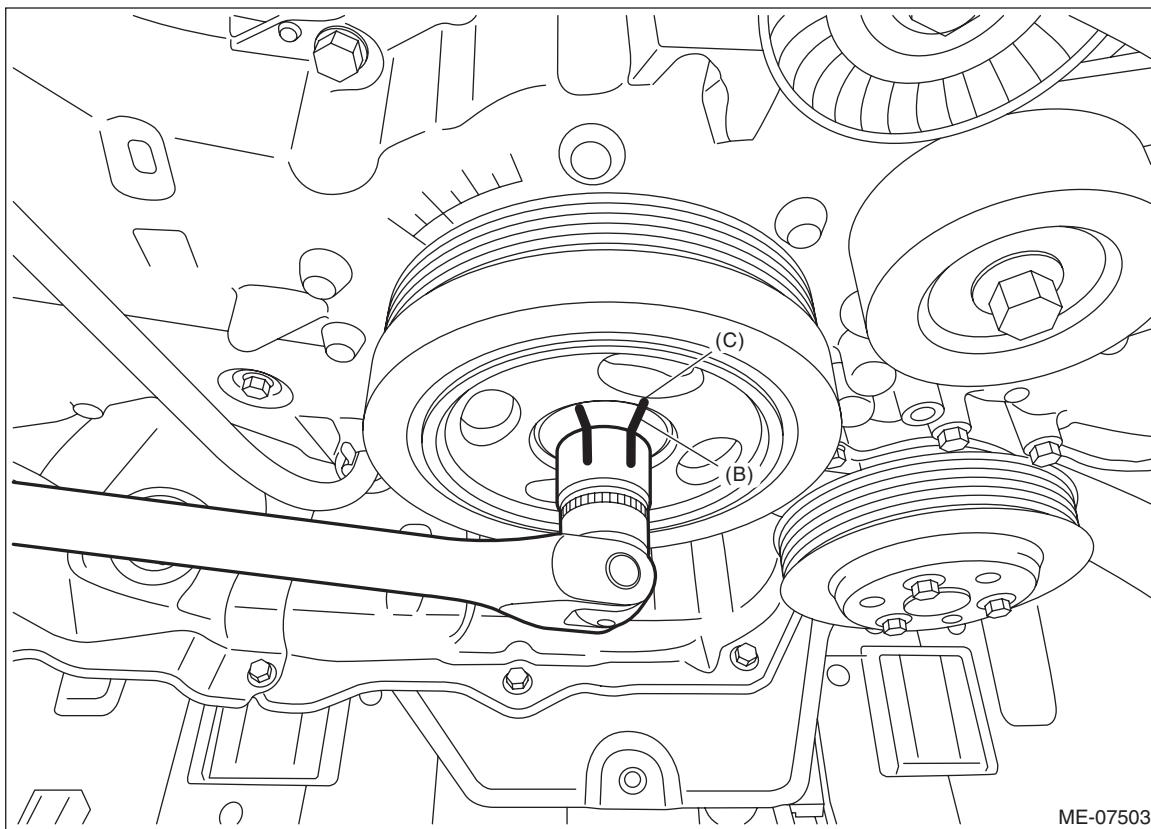
(6) Use the ST to lock the crank pulley, and tighten the crank pulley bolt to the angle where reference line (A) and end line (C) are aligned.
