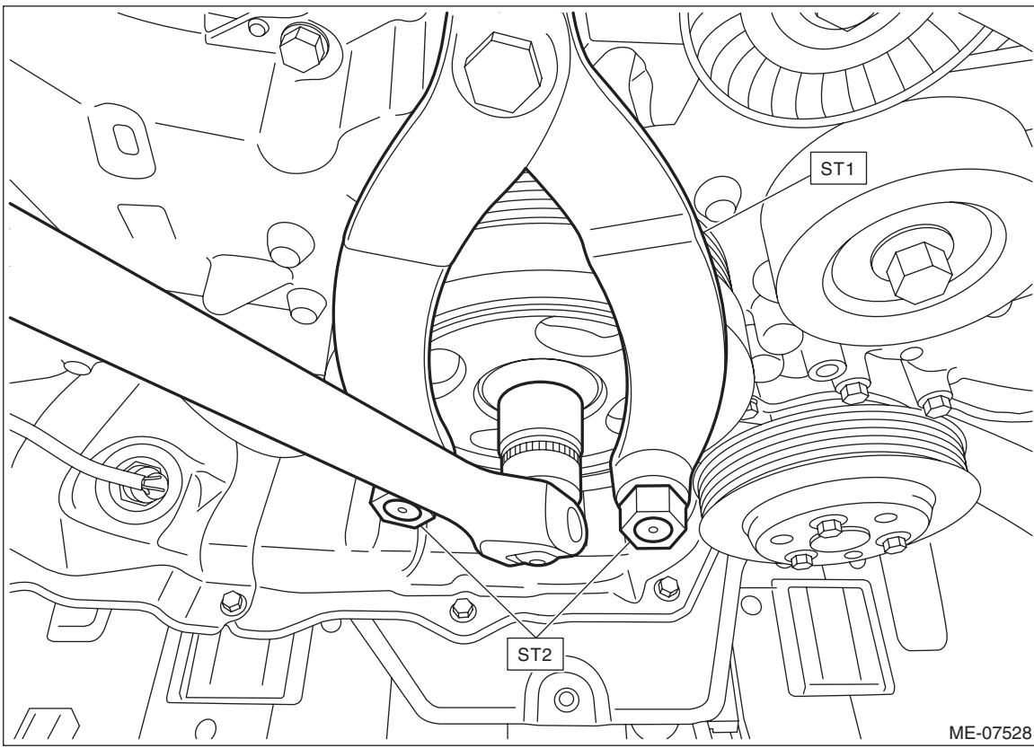
4) Remove the crank pulley.
