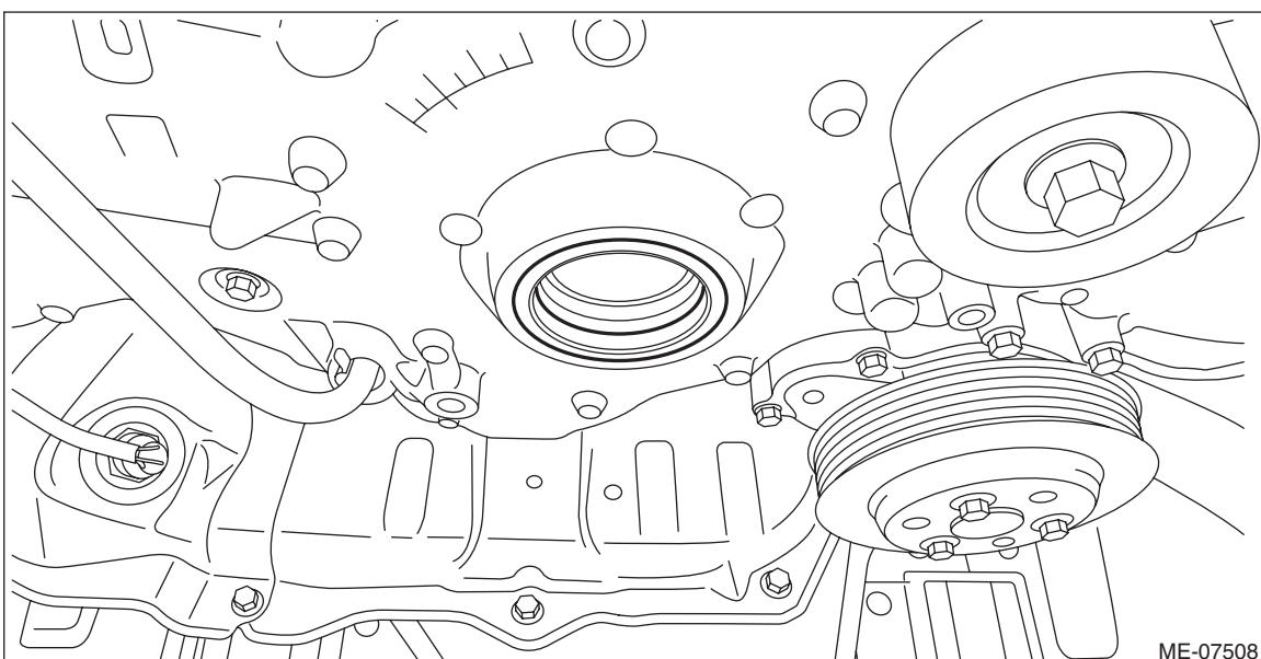
(4) Apply a light coat of engine oil to the front oil seal inner periphery and outer periphery, and install the front oil seal to the chain cover using ST.
