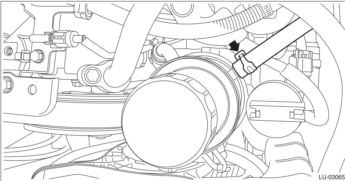
10) Remove the bolt which secures the side engine oil cooler pipe to the cam carrier RH. Remove the side engine oil cooler pipe together with the side engine oil cooler hose A.
