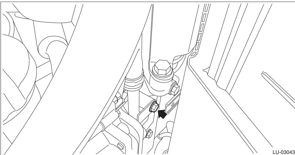
11) Remove the side engine oil cooler hose A from the side engine oil cooler pipe.
