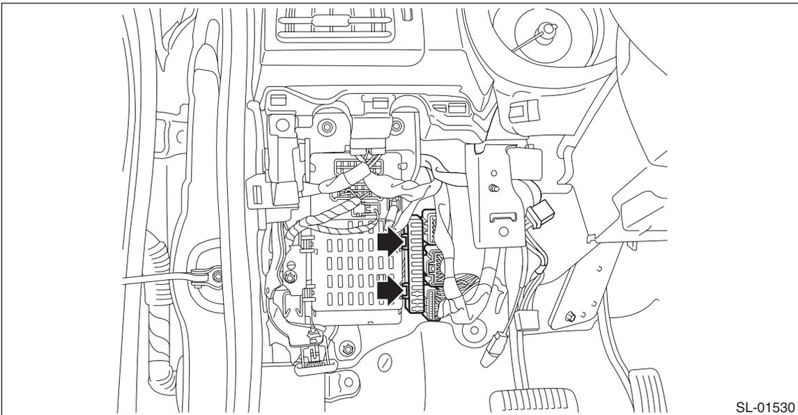
(3) Disconnect the connectors from the relay & fuse box.
