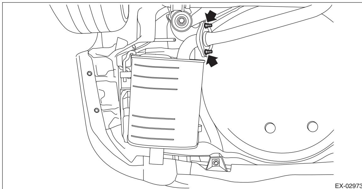
4) Apply a coat of spray type lubricant to the mating area of cushion rubber.
