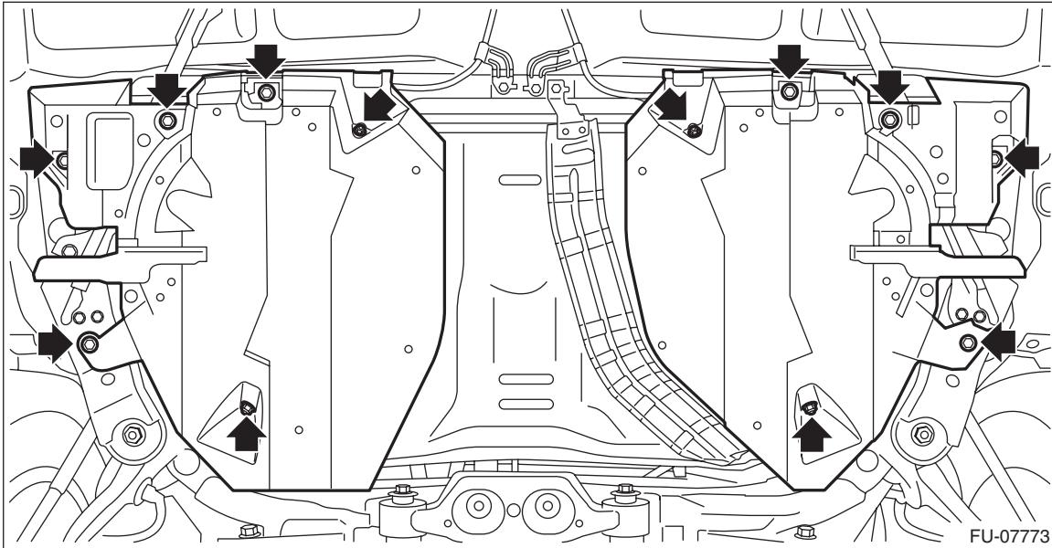
11) Remove the rear sub frame assembly.
