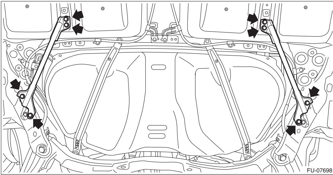
(2) Remove the bolts at the bottom of rear strut assembly.
