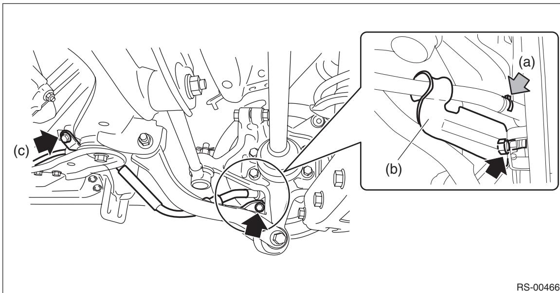
8) Remove the sub rear harness clamp and connector.
